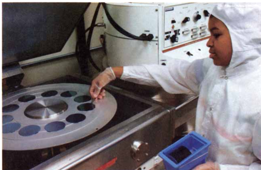
Technician at NCR Corporation Dayton-area microelectronics manufacturing facility places semi-conductor grade silicon wafers in processing equipment at end of cleaning cycle. Hood and smock worn by all employees in area help maintain clean-room standards and reduce chance of inadvertent contamination.
