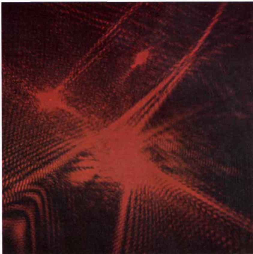
A pattern formed by laser light directed through a sheet coated with glue and plastic strips
