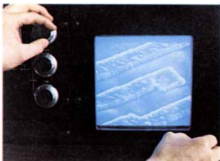
At 10,000X magnification, the details of a VLSI circuit are displayed on the Perkin-Elmer ETEC Autoscan® Scanning Electron Microscope.
