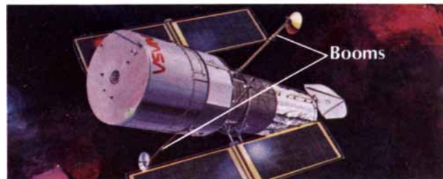
Graphite/Aluminum booms. They have extraordinary strength-to-weight ratios.
