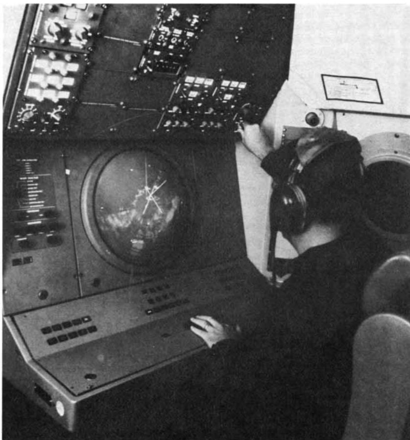
SENSOR STATION NO. 2 on a P-3C Orion antisubmarine patrol aircraft is said to contain the following control and display equipment: radar, electronic surveillance measures, magnetic-anomaly detector and infrared detector (the display part of which is not seen in this view). The photograph and accompanying information were released for publication by the Navy.
