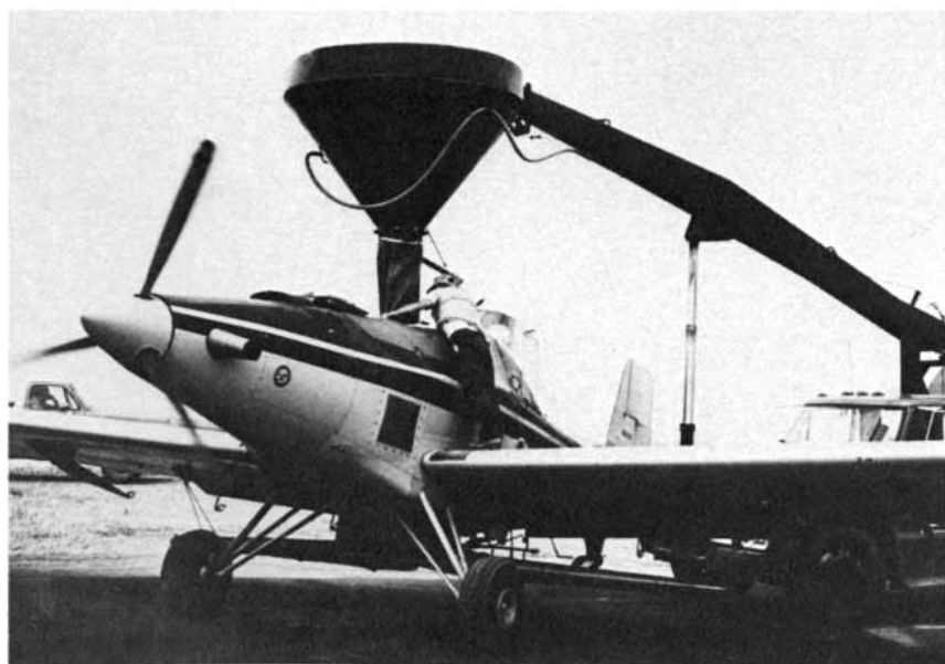
SEED-DISPENSING AIRPLANES such as this one can carry 1,200 pounds of presoaked seed. Presoaking ensures that seed broadcast from the air on flooded fields will sink promptly.
