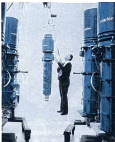
Klystron tubes for UHF television transmitters. Most UHF stations are powered by Varian klystrons.
