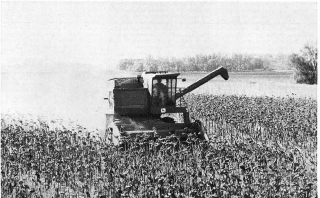
SUNFLOWER CROP IS HARVESTED by a combine. The combine has been adapted to sunflowers by the addition of large metal trays that pass between the rows to catch seeds that fall off prematurely. The trays also guide each stalk into the cutter, which cuts off the
