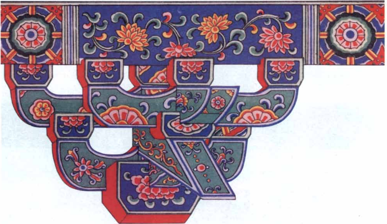
FLORID DECORATION of an identical bracket-arm set, making use of numerous colors, is another of those specified in Li Chieh's
