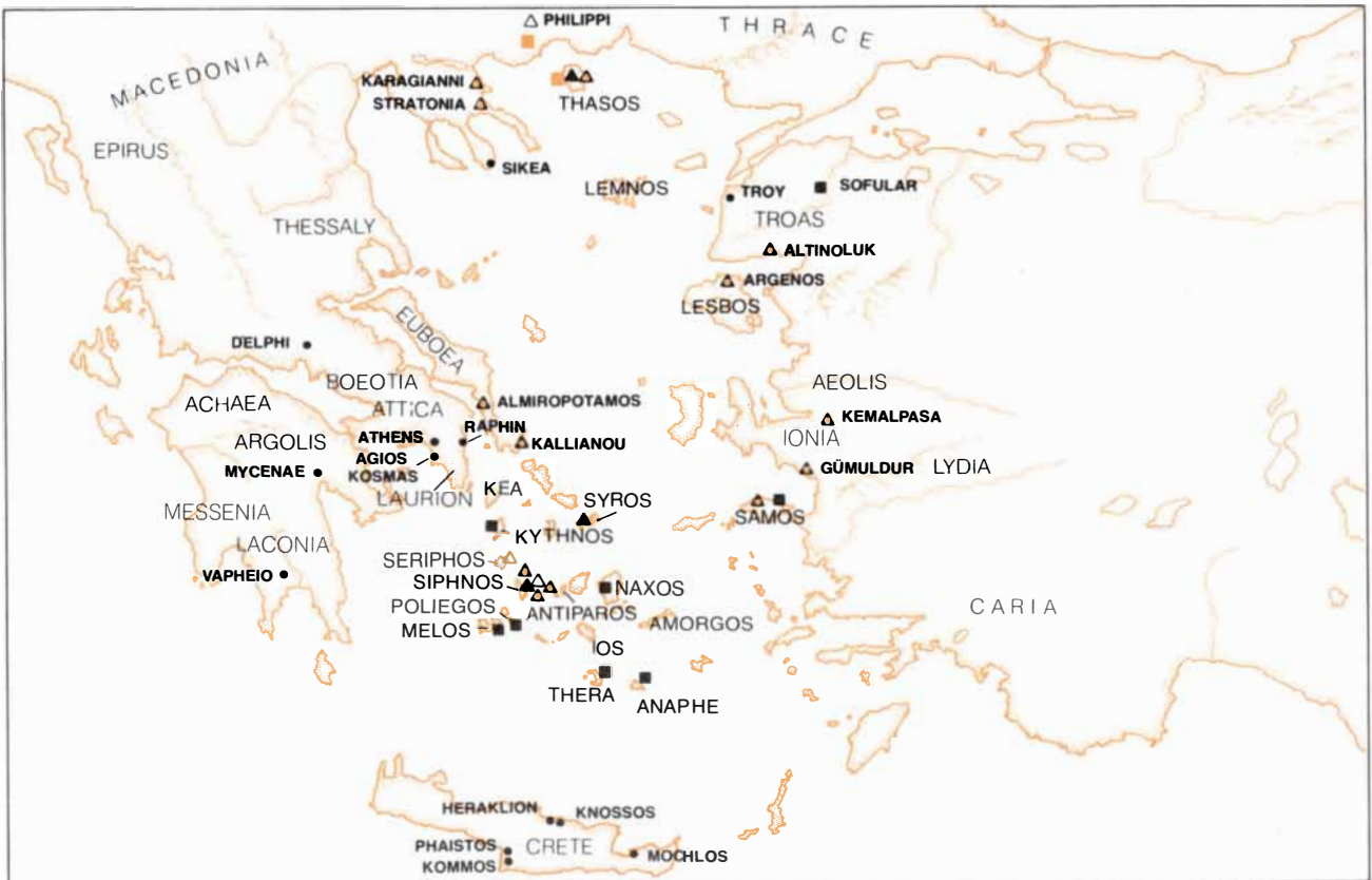
AEGEAN ORE DEPOSITS , many of them unmined in the Bronze Age or in Classical Greek times, are indicated. Black squares designate lead ores and colored squares gold ores. Solid black triangles des-
