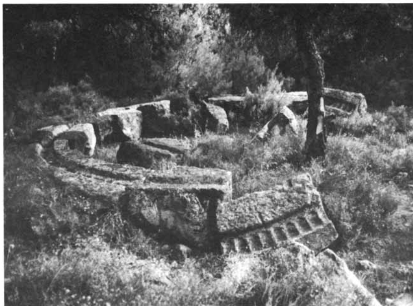
BLOCKS OF MARBLE at Demoliaki in the Laurion once formed a sloping circular sluice some 20 feet in diameter, used in Classical times to separate lead ore from lighter waste rock. The cups cut into the sluiceway retained the heavy ore as a stream of water carried off the waste.
