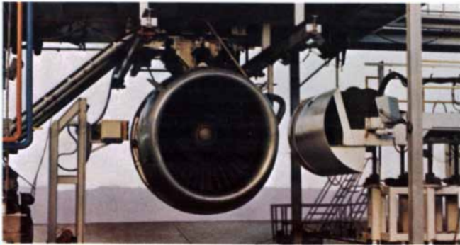
Gas turbine engine under Lockheed X-ray inspection.
