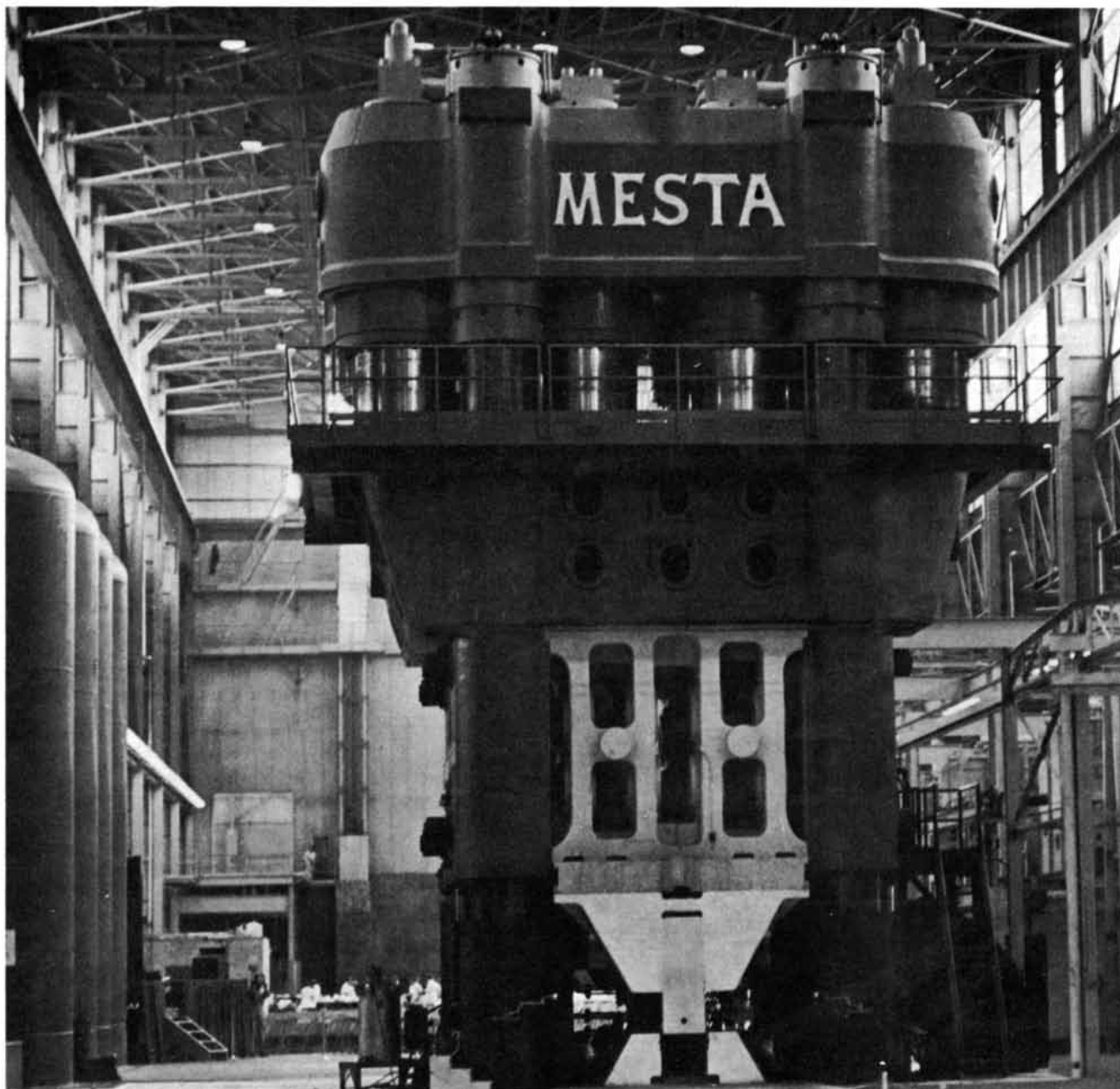
HYDRAULIC PRESS at the Alcoa plant in Cleveland is one of the two largest forging presses in the U.S. It has a capacity of 445 mega-
