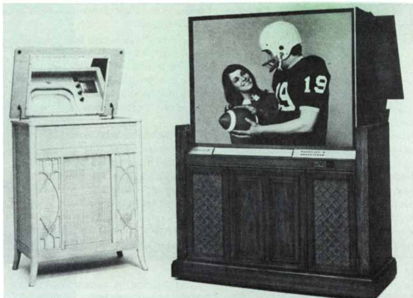
One of the earliest projection TV sets was made over 40 years ago. The experimental model (left) was produced in 1939. The picture tube was over 18 inches in depth, and was mounted vertically in the set. The TV picture was projected up to a mirror in the set's lid. It was then reflected to the viewer, who also saw the controls of the set and the brand name—backwards. Today's equivalent projection color TV set has a 45-inch diagonal screen size. The one-piece unit has the screen concealed inside the cabinet.
