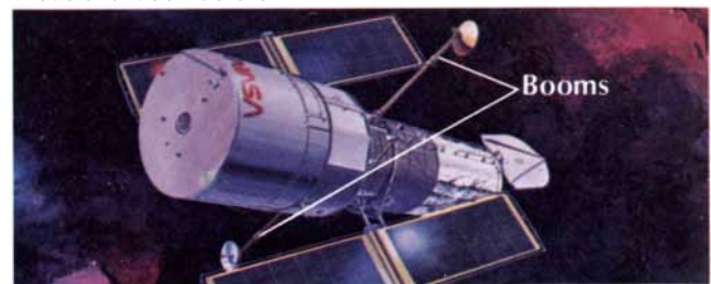
Graphite/Aluminum booms. They have extraordinary strength-to-weight ratios.
