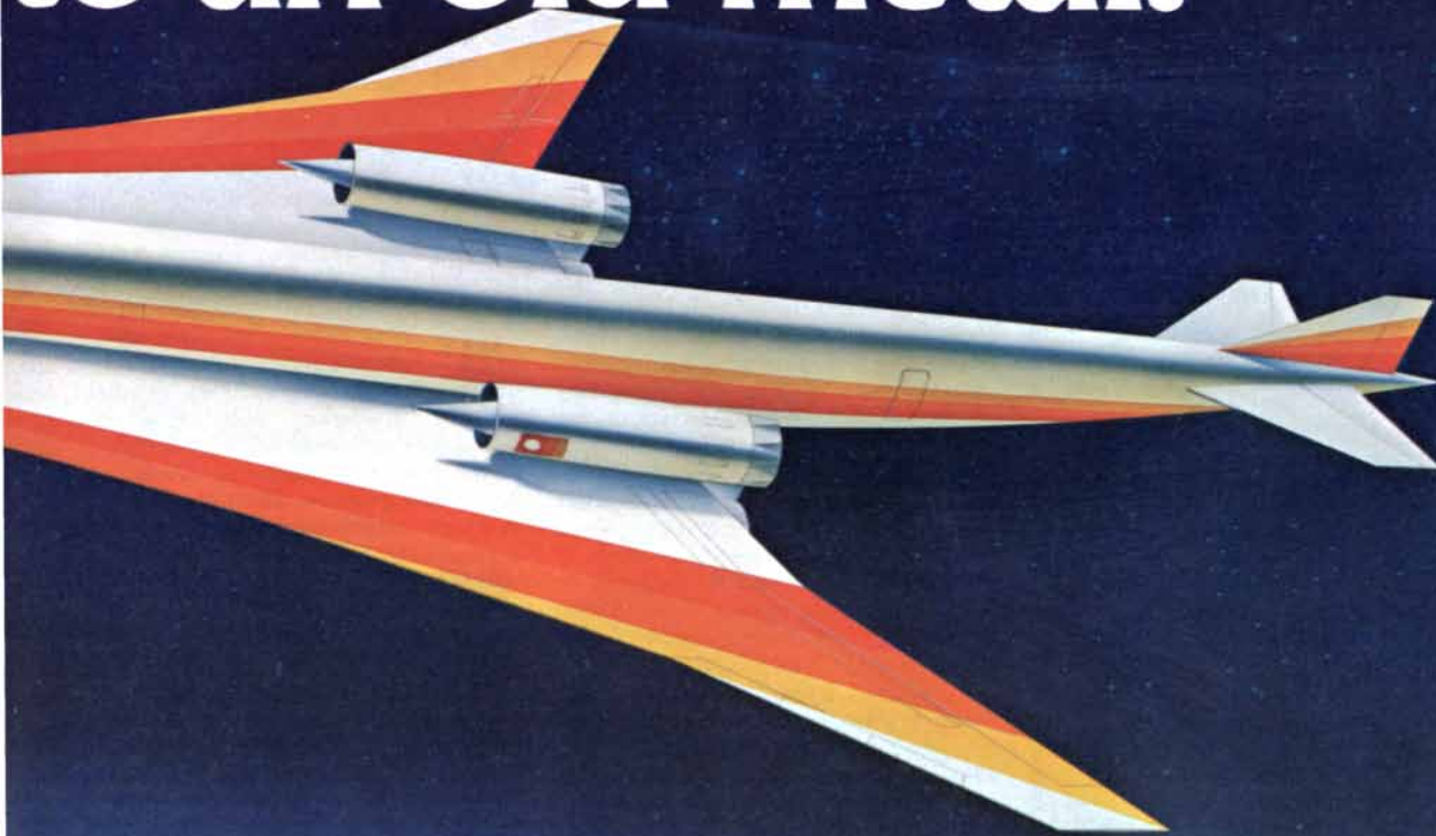
Powdered aluminum would be used in 40% of this advanced jetliner in the 1990's.
