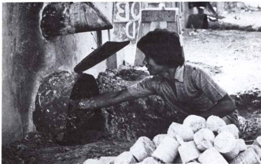
Rice husk briquettes, one of the appropriate technologies developed by the Technology Resource Center, are an economical and efficient substitute for firewood or charcoal.
