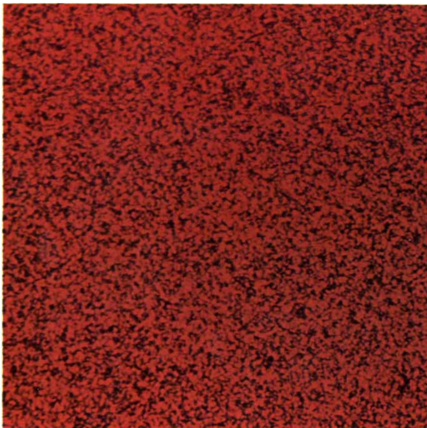
A speckle pattern generated by light from a helium-neon laser
