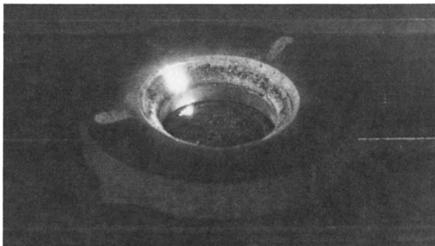
CLOSE VIEW of the valve seat shows the area where the laser beam, which is moved automatically around the surface being alloyed, is delivering its intense heat. The materials being alloyed with the cast iron are in the form of a powder. Because a laser beam does not make mechanical contact with a workpiece the valve seat does not have to be clamped in position.
