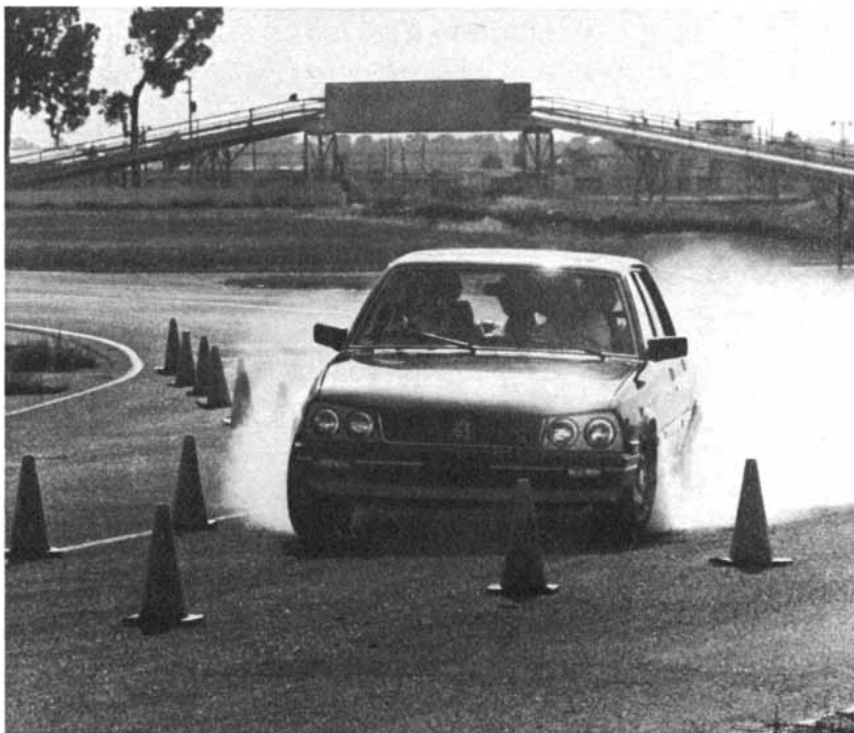
Test driver demonstrates emergency-braking power of Peugeot 505 STI. Driver maintains control, even though car is braking and turning at the same time.
