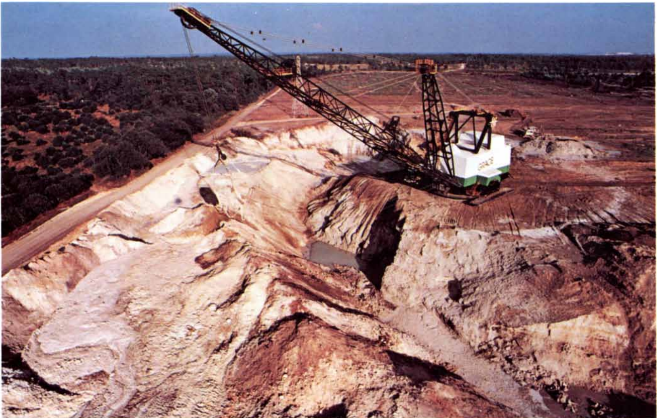
PHOSPHATE IS MINED at one of the large deposits of phosphate rock of marine origin near Bartow in central Florida. The dragline
