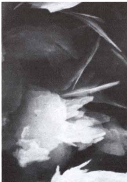
BITS OF PAINT from Lascaux are seen in these scanning electron micrographs. At the left is a red ocher, enlarged 6,000 diameters; the platelike crystals are hematite ( Fe_2O_3 ). At the right is a black manganese, enlarged 7,000 diameters; the needlelike crystals are pyrolusite ( MnO_2 ). The study is being done by Pamela B. Vandiver at the Massachusetts Institute of Technology.
