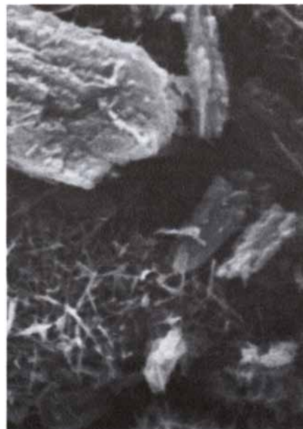
BITS OF PAINT from Lascaux are seen in these scanning electron micrographs. At the left is a red ocher, enlarged 6,000 diameters; the platelike crystals are hematite ( Fe_2O_3 ). At the right is a black manganese, enlarged 7,000 diameters; the needlelike crystals are pyrolusite ( MnO_2 ). The study is being done by Pamela B. Vandiver at the Massachusetts Institute of Technology.
