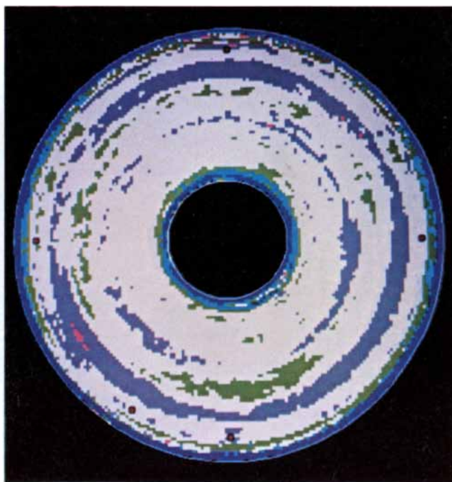
red areas correspond respectively to highs and lows. At the start deviations from the prescribed shape were as great as 100 millionths of an inch; at the finish the maximum deviation was less than a millionth of an inch over most of the surface. The finished primary is the finest large astronomical mirror ever made. According to Perkin-Elmer, "so nearly perfect is the surface that if the mirror were scaled up to the width of the continental United States, no hill or valley would depart from the mean surface by more than about 2½ inches."
