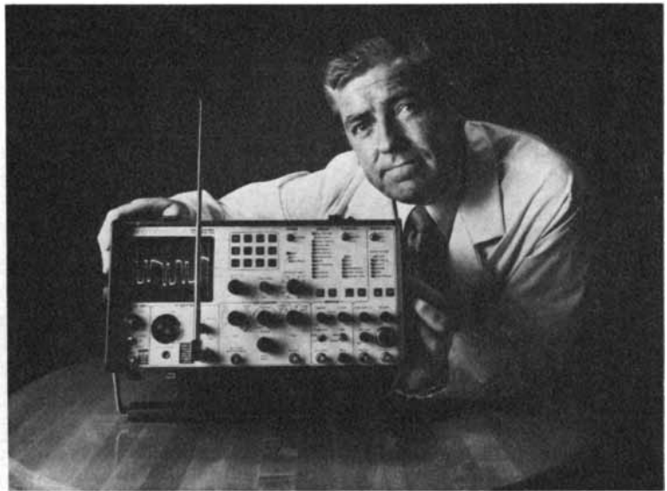
Motorola's R2001. In one "in-the-field" test unit: a signal generator, a frequency modulation, and RF power meter; a spectrum analyzer; a duplex generator, RF memory tables, a code synthesizer, an audio frequency counter, a digital voltmeter, an oscilloscope, and a sweep generator.
