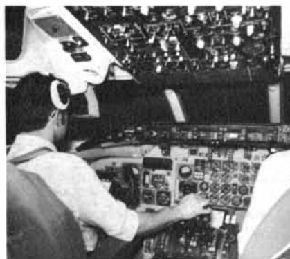
New digital flight guidance and control system has a performance-monitoring capability which helps cut maintenance costs.
