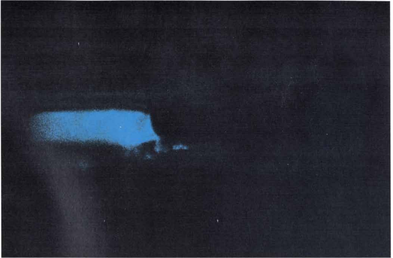
The glow from a wintergreen Lifesaver as it is crushed with pliers
