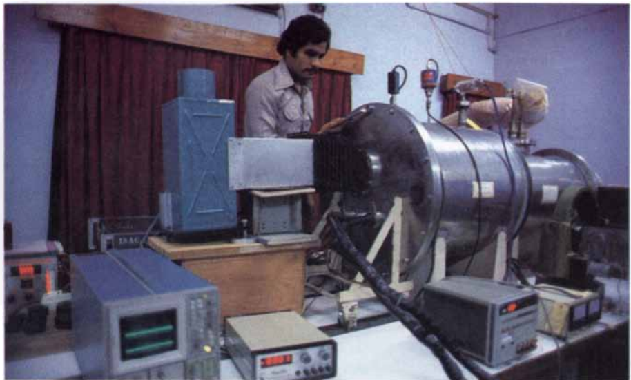
A solid-state satellite camera undergoing thermal vacuum and calibration tests in a space simulation chamber at the ISRO center, Bangalore.
