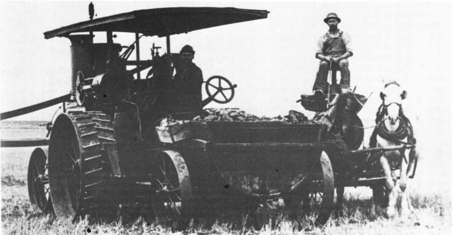
belt. The separator removed the grain from the stalks. Five horses (of the 10 or so needed in the operation) and 13 men can be seen. Most of
