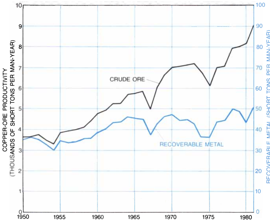
PRODUCTIVITY IN COPPER-ORE MINING between 1950 and 1981 increased at a rate of 3 percent per year on a crude-ore basis (black curve) and at a rate of 1.2 percent per year for recoverable metal (color). About 85 percent of the copper-ore tonnage is extracted from open-pit mines. In 1950 each ton of copper ore mined contained an average of about 19 pounds of copper. By 1981 the average metal content had dropped to about 11 pounds per ton of ore.
