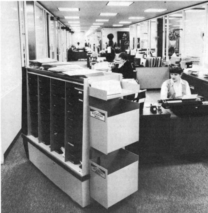
MAILMOBILE , a driverless battery-powered delivery vehicle made by Bell & Howell, mechanizes intraoffice deliveries. Here it is negotiating a curve as it makes its way through the research department of Merrill Lynch and Company. The vehicle follows a chemical pathway, which is easily applied and modified to trace any route from the mail room through the office and back to the mail room. An emitter of ultraviolet radiation under the vehicle makes the chemical fluoresce; an optical sensor detects the fluorescent path. The Mailmobile moves at about one and a half feet per second (one mile per hour), beeping and flashing blue headlights. It stops at pickup and delivery sites designated by a coded pattern in the chemical pathway. Bumpers stop the vehicle on contact with a person or another obstacle. An "intelligent" version is being introduced that can be directed to choose among alternate paths or to board an elevator.
