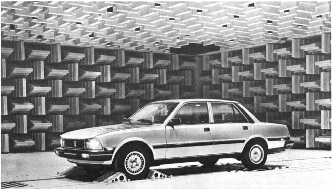
From Europe's second-largest carmaker comes the Peugeot 505S, seen here undergoing silence tests in the soundproof chamber.
