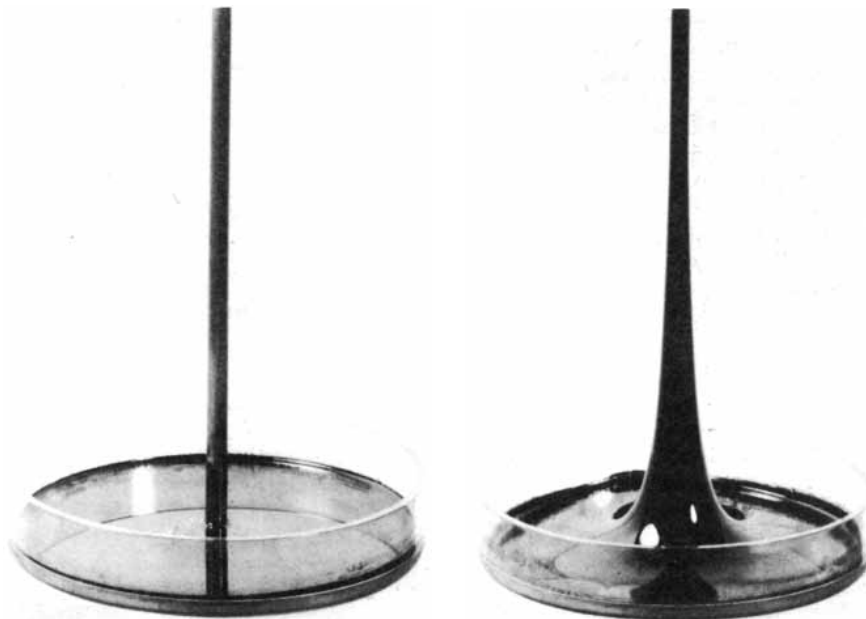
BALANCE OF MAGNETIC AND GRAVITATIONAL FORCES is demonstrated when an electric current is passed through a metal rod placed upright in a pool of ferrofluid. The photograph at the left shows the experimental arrangement in the absence of current. When the current is turned on, the fluid leaps upward, as shown in the photograph at the right. At each point in the ferrofluid the sum of the magnetic, gravitational and pressure energies is constant.
