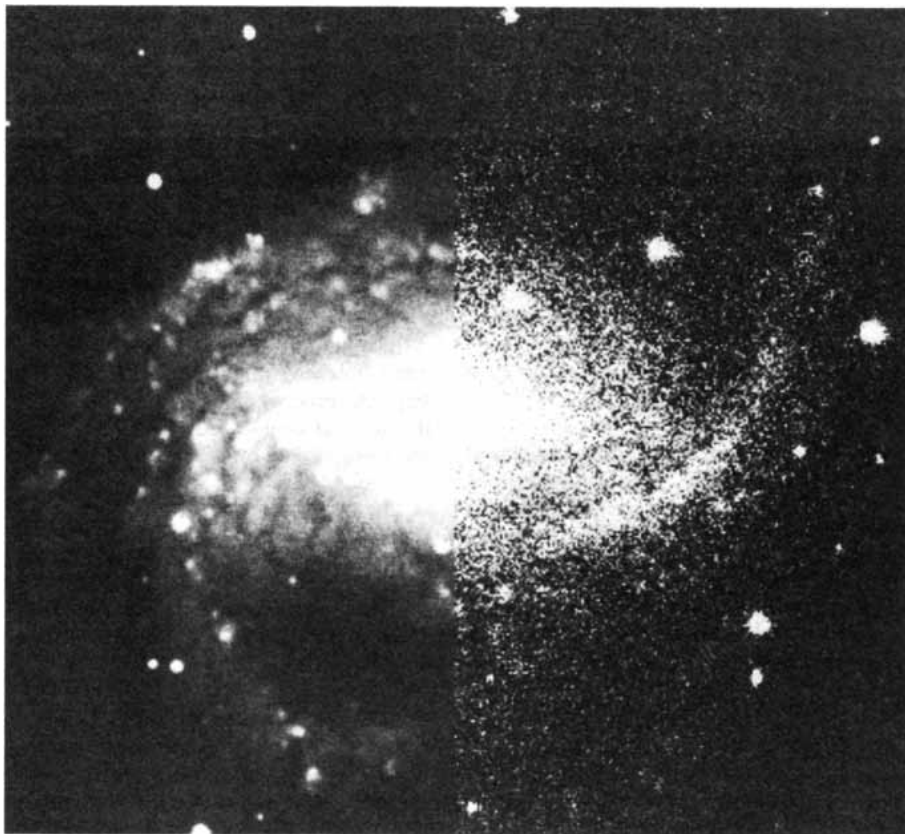
EFFECT OF NOISE on a CCD image is demonstrated in this mosaic picture of the bright spiral galaxy NGC 6951. The clarity of the original short-exposure image ( left ) is limited by "photon noise" (that is, random fluctuations in the number of photons striking the detector). In the right half of the picture the noise level of the original image has been artificially increased by computer processing but the image is otherwise unchanged. The most obvious effect of the added noise is an appearance of increased granularity. On closer inspection the loss of information in the altered image is evident in the reduced visibility of fine details and of low-contrast features such as H II (ionized hydrogen) regions and dust lanes in the galaxy's spiral arms.
