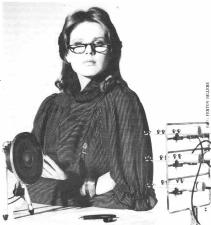
Latest sound intensity probes array for in situ measurement of acoustic power and directivity pattern of industrial noise sources.
