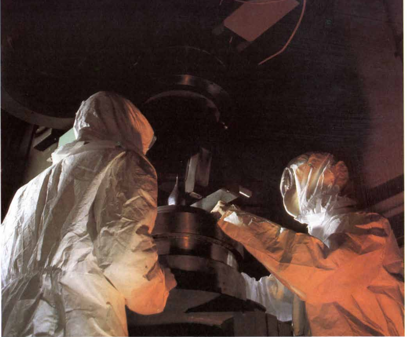
Production of gallium arsenide monocrystals, 75 millimeters in diameter, which are used for key components required for the Thomson group's electronics products.
