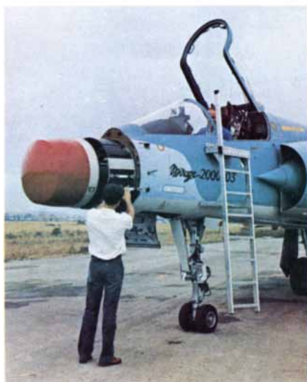
The Thomson-CSF "RDM" multirole radar being fitted on a Dassault Mirage 2000.
