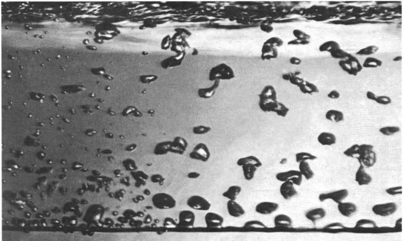
John H. Lienhard's photograph of acetone boiling in two stages over a heated wire: nucleate boiling (left) and film boiling (right)
