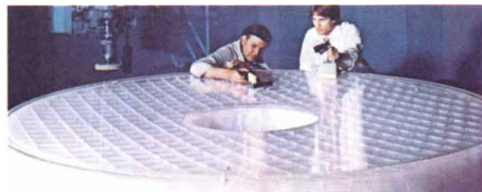
The extremely smooth, precisely shaped primary mirror surface will result from two full years of grinding and polishing.
