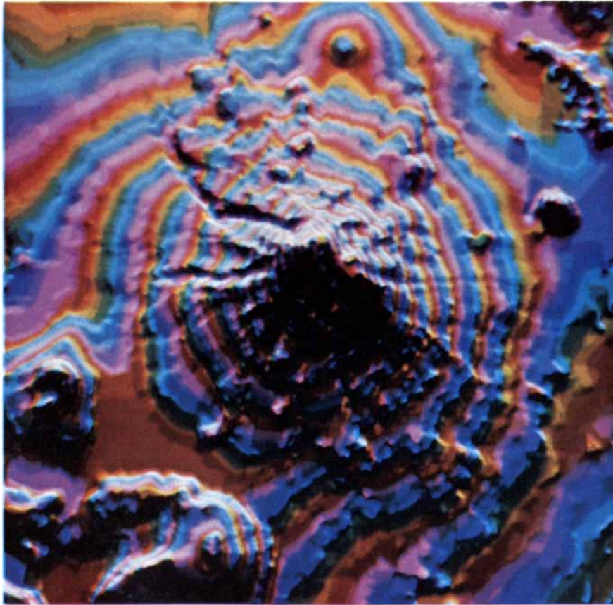
SIMULATED RADAR IMAGE of Mount Shasta in northern California was prepared by Michael Kobrick of the Jet Propulsion Laboratory in the course of investigating the feasibility of gathering three-dimensional information about the earth's surface by means of a spaceborne radar interferometer. In such a system the phase difference between the microwave echoes received by two antennas mounted on the same spacecraft would be measured on a point-by-point basis to generate a topographic image. Here the topographic data were actually obtained first by conventional means and then processed to simulate the digital output of an orbiting radar interferometer. The multicolored topographic contours derived from the resulting stream of digital information correspond to lines of constant height above sea level.
