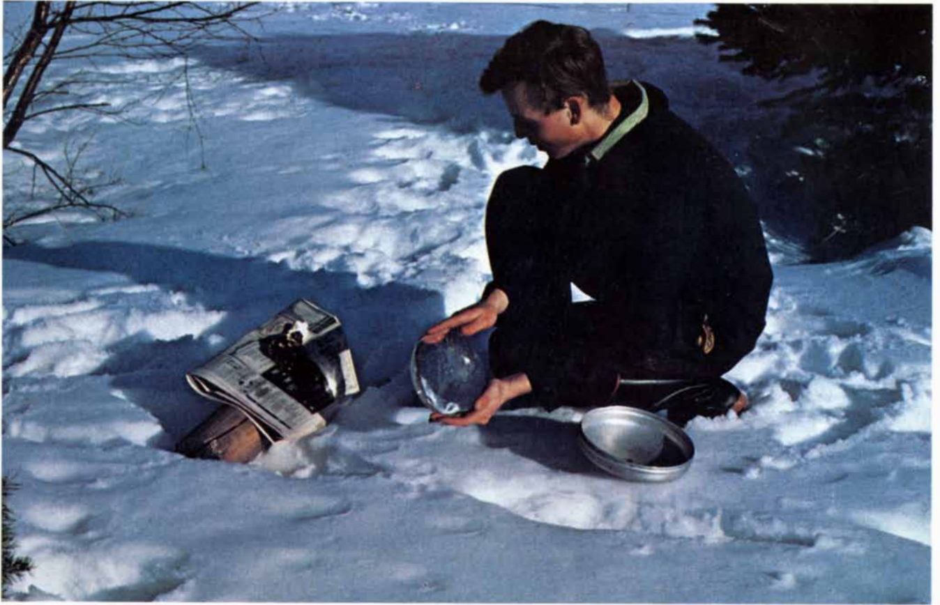
Matthew G. Wheeler employing one of his ice lenses to ignite paper
