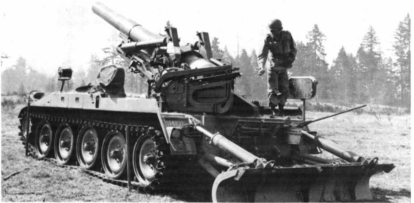
U.S. M110 203-MILLIMETER GUN is shown being test-fired with a non-nuclear shell. The eight-inch howitzer is also capable of firing a nuclear shell. Its maximum range is approximately 16 kilometers.
