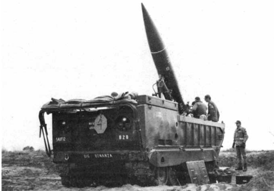
U.S. LANCE MISSILE is seen being readied for a test launch from its self-propelled erector-launcher vehicle. The liquid-fuel rocket can carry either a nuclear warhead or a conventional one. Its maximum range is about 115 kilometers. The Lance has replaced the Honest John as the standard U.S. battlefield nuclear missile. Other NATO nations have both the Lance and the Honest John in their arsenals. All nuclear warheads for the missiles are in U.S. custody.
