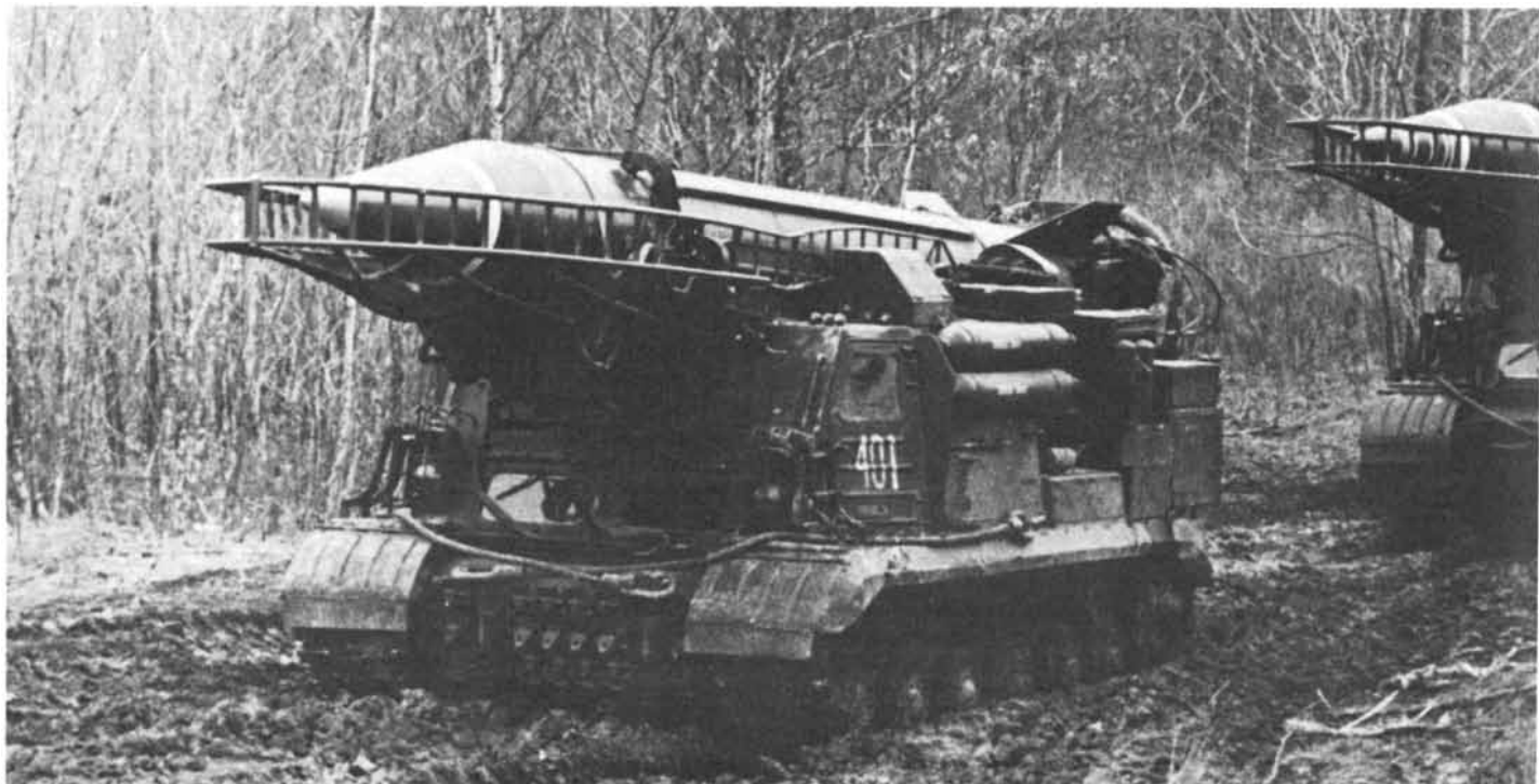
RUSSIAN SHORT-RANGE MISSILES are transported across a muddy field on tracked erector-launcher vehicles. The missiles, des-
