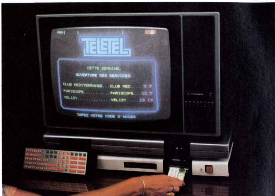
The smart card is used for telepayment or teleshopping simply by inserting it into a minitel terminal. The home user places the card—with a microprocessor and memory embedded in it—into an add-on card reader/processor and, after typing a personal identification number, the memory written into the card by the issuing authority identifies the user, indicates the money value or banking power of the card and automatically dates and records information within the integrated circuit. The card can be used for a variety of other banking and business applications.
