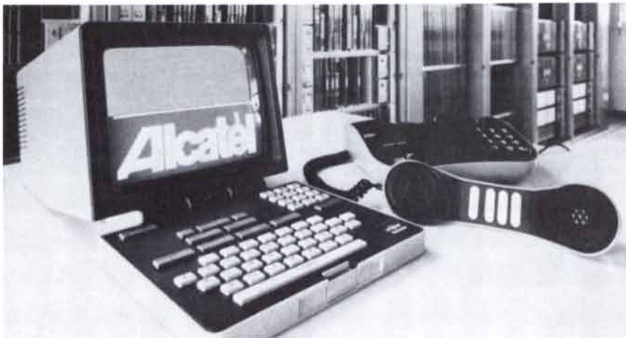
A CIT Alcatel minitel videotex terminal in the foreground of the E 10-Videotex switching system is an example of the adaptability of the E 10 to new telecommunications requirements. The unit provides the interface between the subscriber and the data bank, controls the connection, and handles format, transmission speed, and signaling conversions.
