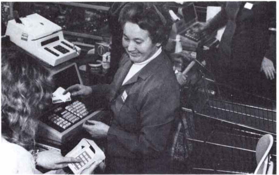
The public point-of-sale test in Saint-Etienne uses a multiservice terminal and credit cards with magnetic stripes to interact in real time with a central computer over the French packet-switched data network. The user is providing the system with her personal identification code.
