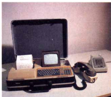
Numerous small French companies are active in telecommunications. This portable minitel terminal is manufactured by FIET.
