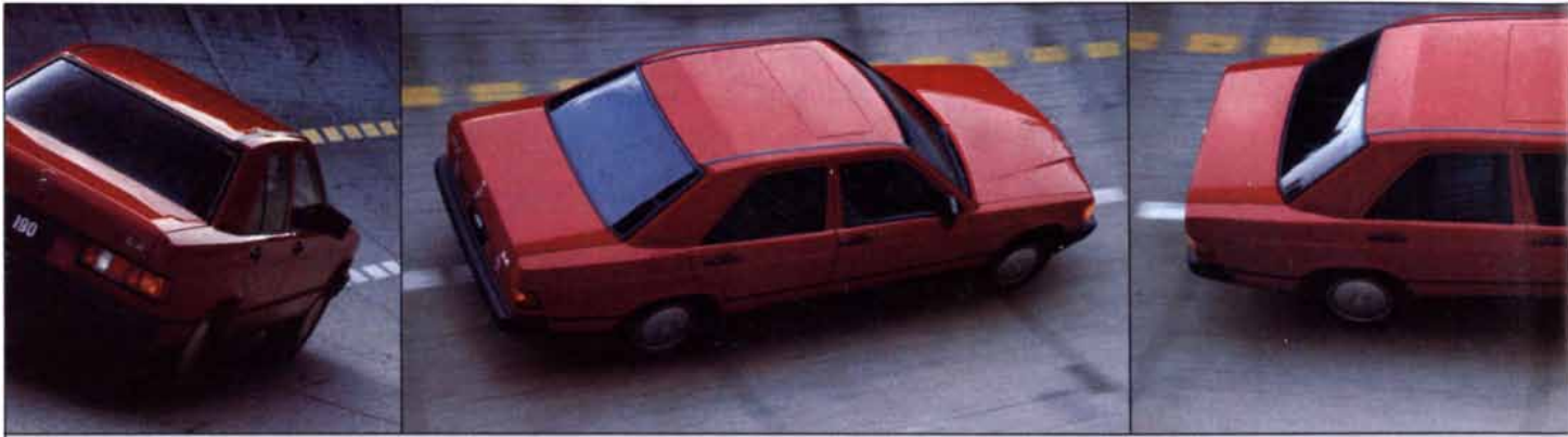
The new 190 E 2.3 Sedan: a $24,000* four-door wedge that weighs 2,655 lbs., has an aerodynamic drag coefficient of 0.35,
