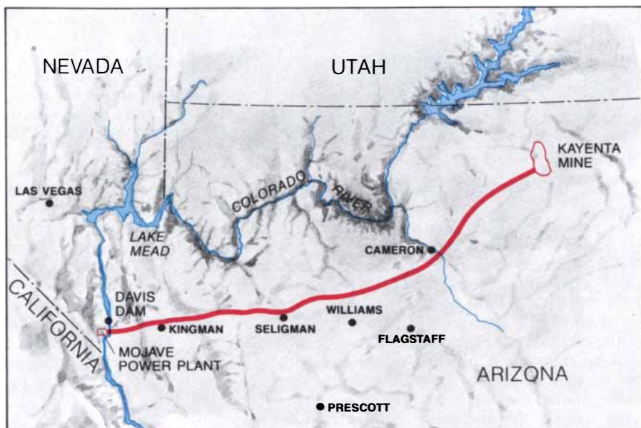
LONGEST SLURRY PIPELINE currently in operation is the Black Mesa line of Southern Pacific Pipelines, Inc. It moves coal 273 miles from the Peabody Coal Company's Kayenta mine in Arizona to the Southern California Edison Company's Mojave power station in Nevada. For most of its length the pipeline is 18 inches in diameter. The Black Mesa line carries 5.5 million tons of coal per year with 99 percent reliability. It went into operation in 1970.
