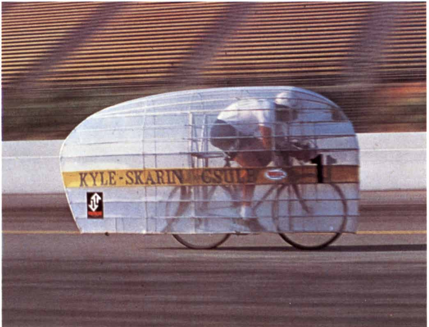
STREAMLINED RACING BICYCLE designed by one of the authors (Kyle) and ridden by Ronald P. Skarin, an Olympic cyclist for the U.S., is shown setting the world record of 31.88 miles per hour for one hour of pedaling from a standing start. The key to the perform-
