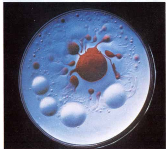
Frode Wissing's experiments in which a drop of oleic acid consumes paraffin drops on water
