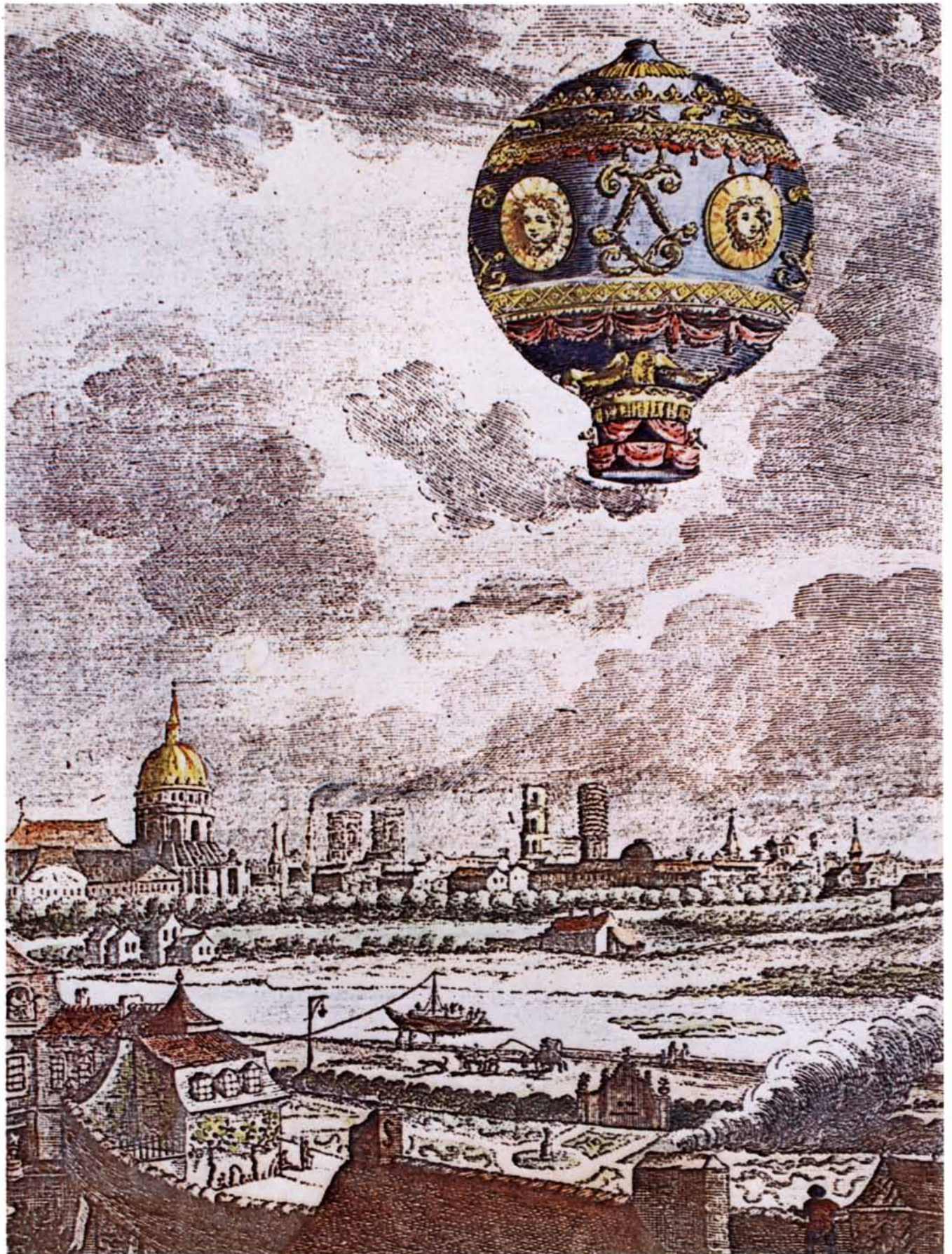
FIRST FREE FLIGHT of a manned hot-air balloon took place over Paris on November 21, 1783. The elaborately decorated balloon, designed by the Montgolfier brothers, was 46 feet across and 70 feet
