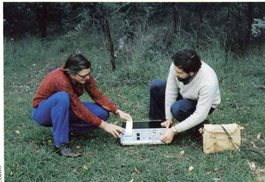
CSIRO's Sirotem, a computerized direct digital borehole logging system and data processing center, can detect ore bodies covered by thick layers of conductive material.
