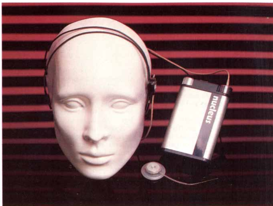
The complete cochlea implant system including implantable prosthesis microphone headset and speech processor.
