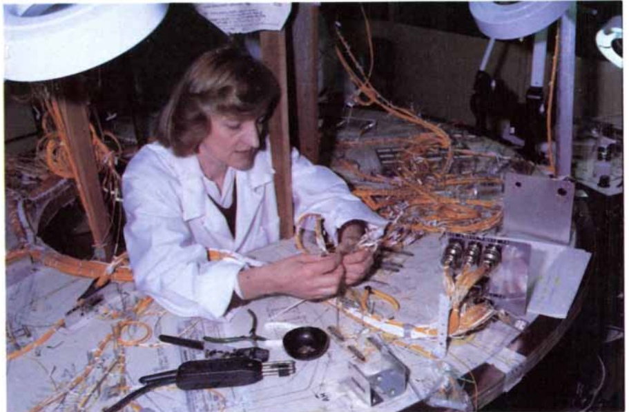
An Australian technician assembling components for AUSSAT's satellites. Sydney, NSW.
