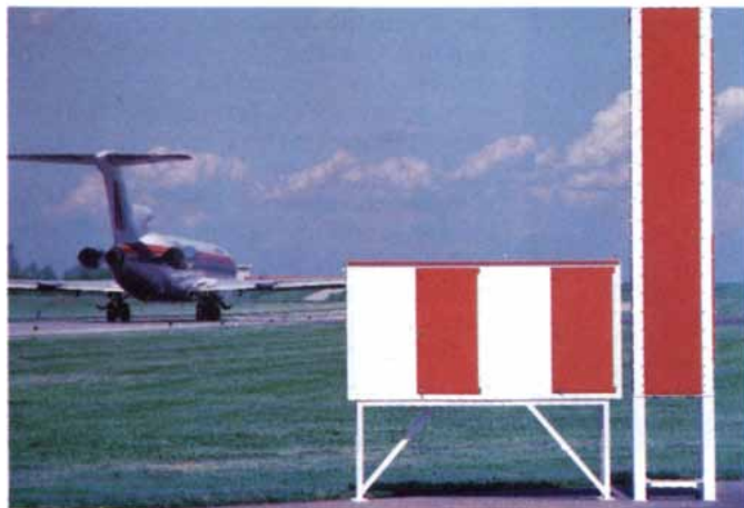
The Interscan microwave landing system. The 1½ degree elevation antenna and associated electronics cabinet on display at Kansas City International Airport (left); the scanning principle (right).
