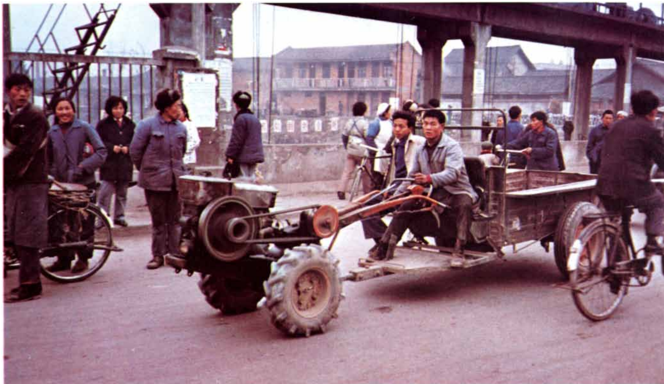
CHINESE FARM MACHINERY appears primitive by the standards of the economically developed countries but has reduced the demand for labor on the collective farms. The photograph was made by the author in the province of Sichuan during a visit to China in 1982. The front of the vehicle shown is a gasoline-powered unit that
