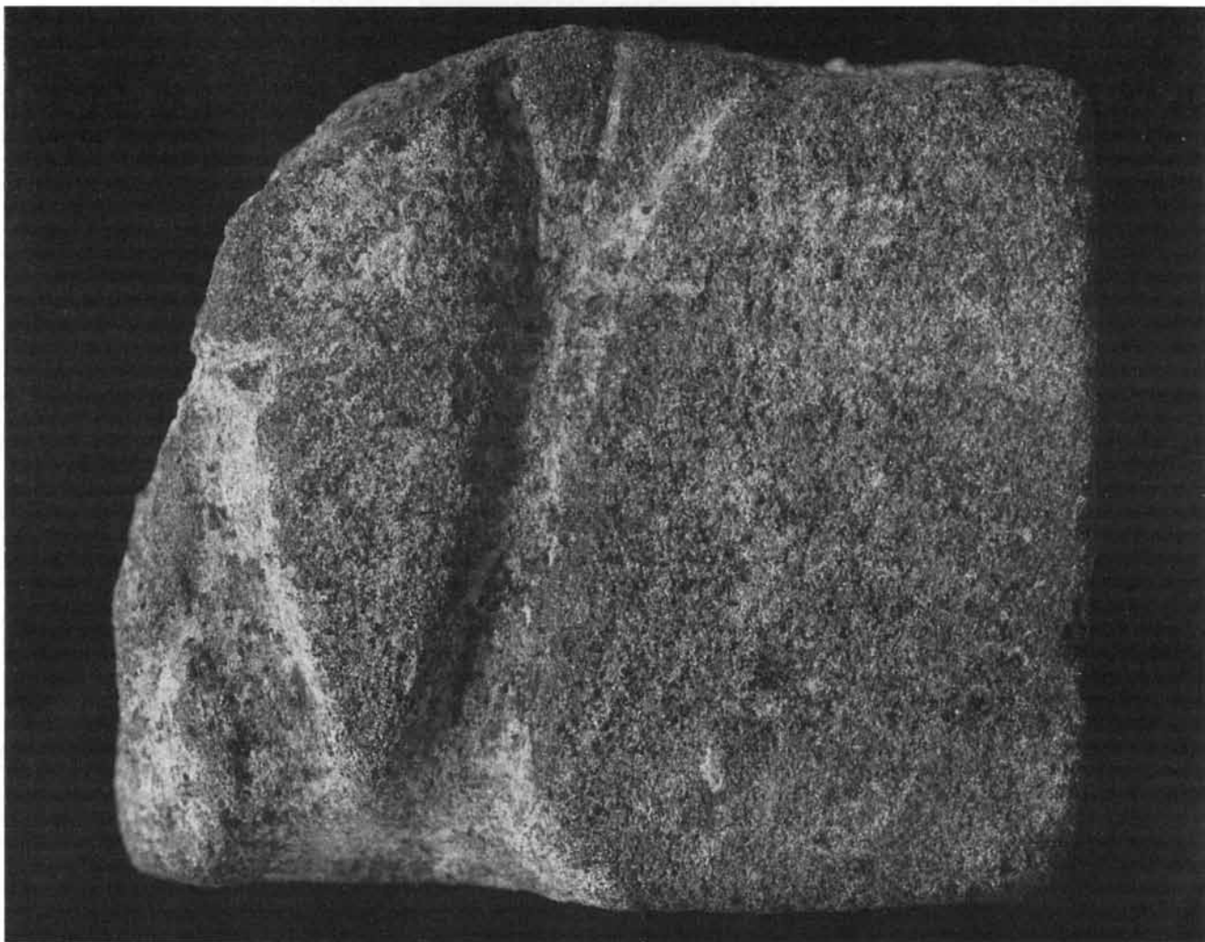
SANDSTONE FRAGMENT is part of a mold used by the Ban Na Di metalsmiths to form a lead replica of a bronze object. When the
