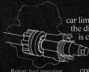
Rotary fuel injection pump precisely measures fuel for each cylinder
