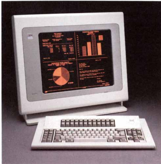
Figure 1. The IBM 3290 Information Panel uses alternating current (AC) plasma technology, making possible high information content and distortion-free images. The screen, which is 10.7 inches by 13.4 inches, can display up to 10,000 characters and can simultaneously display four applications from one or more computers. Its great versatility allows it to mix graphics, images, and text.
