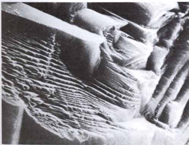
SCANNING ELECTRON MICROGRAPHS of peridotites from oceanic fracture zones show how they can be altered by contact with seawater. The peridotite at the left is from the Red Sea. It is unaltered. The surface of a crystal of pyroxene is stepped by a series of cleavages. The peridotite at the right is from Romanche. It is greatly
