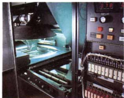
Figure 3. The proximity printer shown here is one of many tools developed by IBM to mass-produce the AC plasma display panel. This machine automatically prints the hundreds of conductor lines on the glass plate by using highly collimated light to expose the conductor pattern through a mask. This projection printing system produces an excellent image and lowers the number of defects.
