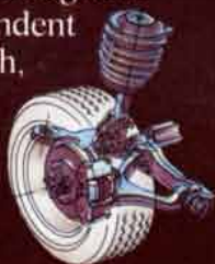
Four-Wheel Independent Suspension
