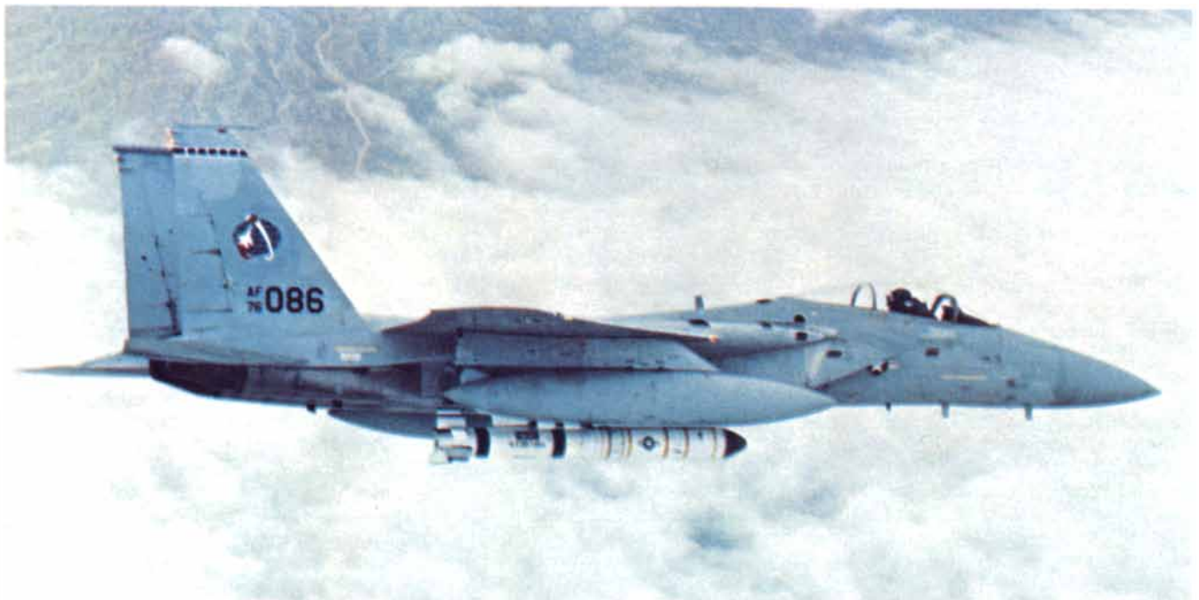
U.S. ANTISATELLITE WEAPON is designed to be launched into space from an F-15 fighter plane at high altitude. The two-stage booster rocket carrying the miniature homing vehicle is seen here
