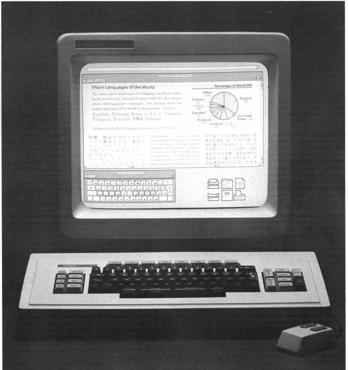
COMPUTER WORK STATION includes the screen whose content was shown in the illustration on the preceding page. The computer itself is part of a computer system called Star manufactured by the Xerox Corporation. The space bar on its keyboard is actually four space
