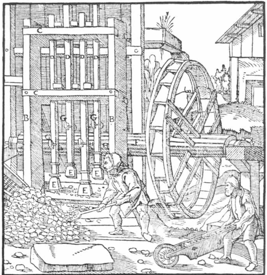
CAM PRINCIPLE WAS APPLIED in a rock-crushing mill illustrated in De re metallica . Cams on the axle engage and then release a tappet (g) attached to each of the iron-shod stamps.
