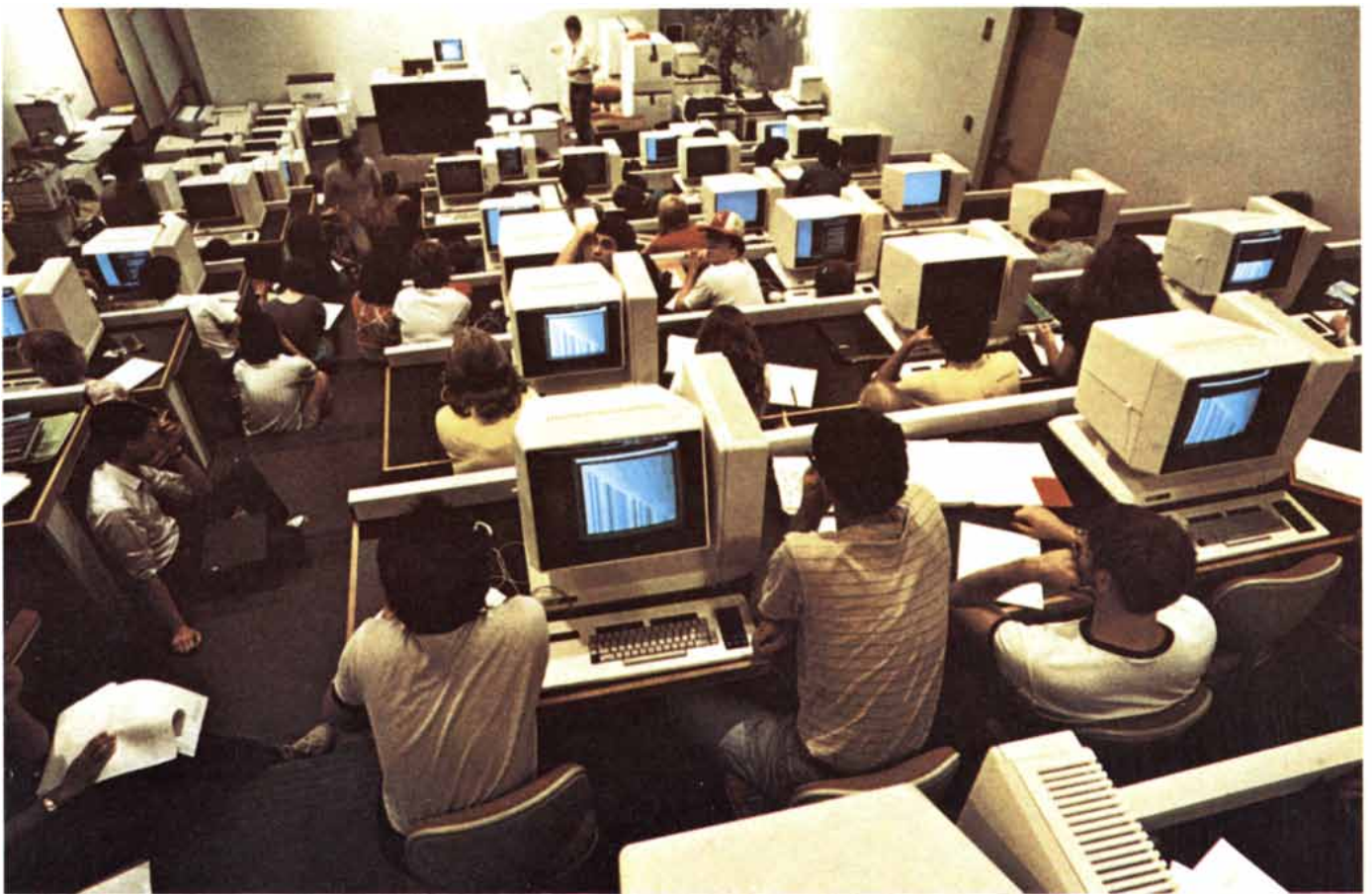
ELECTRONIC CLASSROOM developed by Robert Sedgewick and the author together with their colleagues in the computer-science department at Brown is equipped with 55 high-performance work stations connected in a high-speed network. The instructor can first pre-
