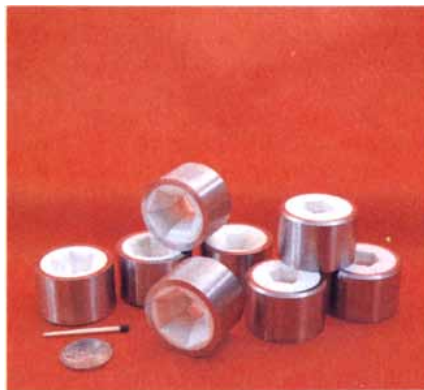
Shaped hot brass rod extrusion
