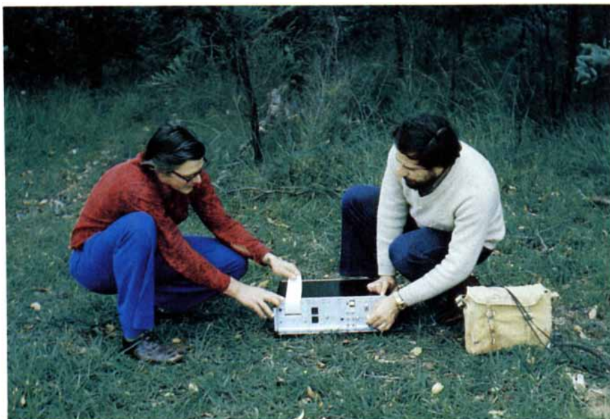
CSIRO's Sirotec, a computerized direct digital borehole logging system and data processing center, can detect ore bodies covered by thick layers of conductive material
