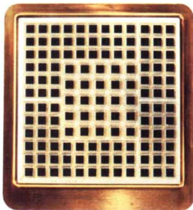
Figure 1: The logic module used in large IBM computers (cutaway below) is part of the industry's densest circuit packaging. The electronic chips mounted in each module (right) were made through IBM's Engineering Design System and the masterslice concept: customize where necessary, standardize where possible.
