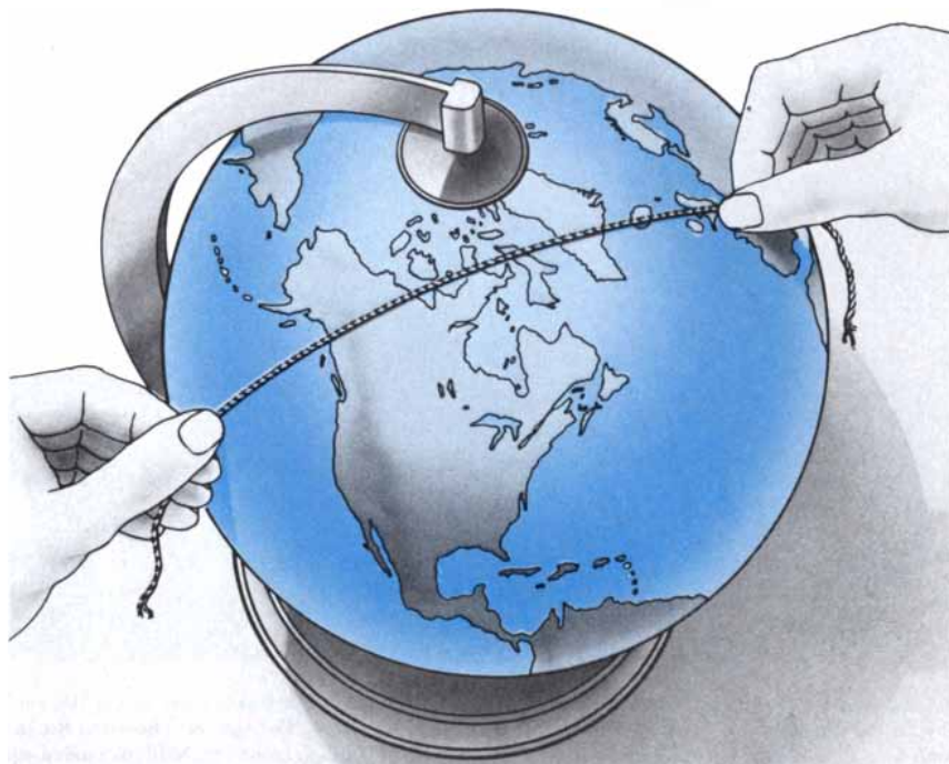
GEODESIC ON A SPHERE is the shortest distance between two points that can be measured on its surface. On a globe a geodesic is the shorter arc of the great circle that passes through the two points. It can be determined by holding a taut string between the points.
