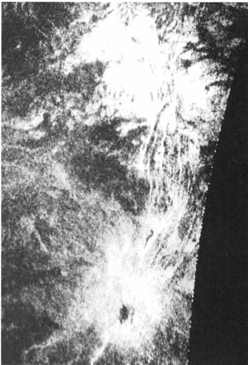
RADAR IMAGE OF BETA REGIO suggests that Theia Mons and Rhea Mons are shield volcanoes flanking a linear rift in the crust. Made at 12.6-centimeter wavelength with the 300-meter radio telescope of the Arecibo Observatory, the image represents variations in surface roughness: bright areas are relatively rough and unweathered, dark areas are relatively smooth. Theia is the circular feature at the bottom of the image; its brightness is attributed to geologically recent lava flows. The linear features running north to Rhea are thought to be a rift, in part because they parallel a canyon discovered in topographical studies. The pattern suggests regional upwelling has lifted the crust in Beta, producing the rift and the volcanoes. The image has a horizontal resolution of approximately two kilometers.
