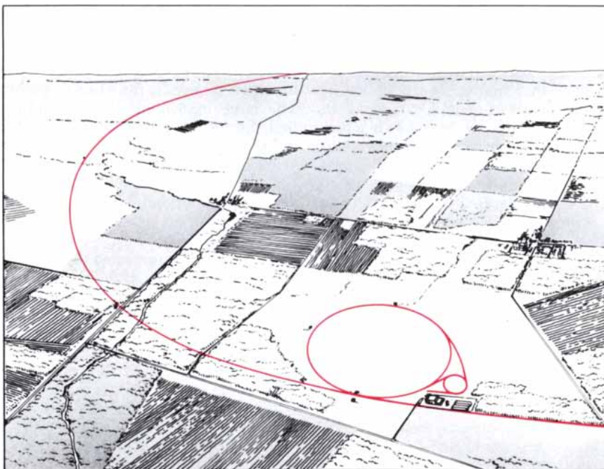
PROPOSED ACCELERATOR , the Superconducting Supercollider, will make it possible to study interactions at energies of more than 1 TeV. In the design depicted (one of many) the accelerator ring has a diameter of 30 kilometers and is buried 100 meters underground; smaller rings feed protons into the large ring. A cross section of the main tunnel ( above ) shows the two pipes, each about five centimeters in diameter, which will contain the counterrotating beams of protons. Superconducting magnets supercooled with liquid helium to increase their power and efficiency surround each of the pipes, focusing and confining the beams.
