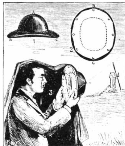
A camera obscura made from a derby
