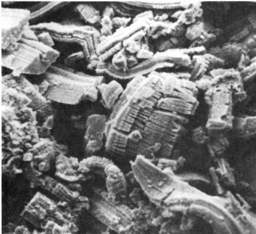
VERMIFORM KAOLINITE , enlarged 1,350 diameters in a micrograph made by Keller, was formed by weathering. Such clays are conceivable two-dimensional genetic crystals.
