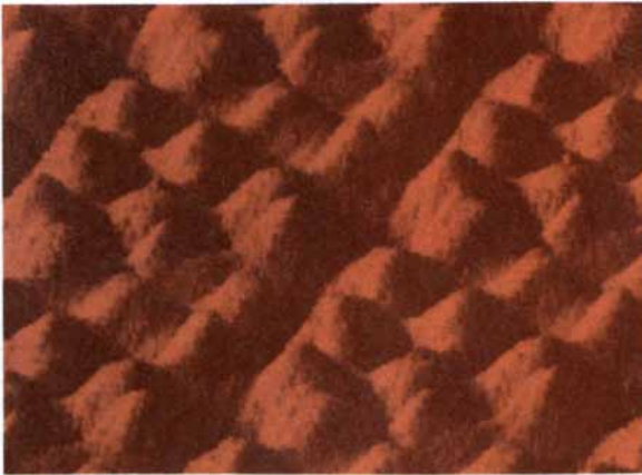
Figure 1. This three-dimensional representation of a silicon surface was obtained by scanning tunneling microscopy, developed by IBM. The individual hills or bumps indicate actual atoms separated by as little as six angstroms. (One angstrom is one ten-billionth of a meter.)
