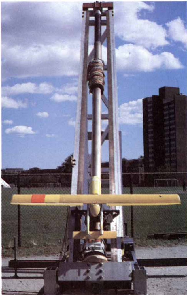
Coilgun (left) can propel glider to a speed of 150 miles per hour; schematic diagram of railgun (top right) and of coilgun (bottom right)
