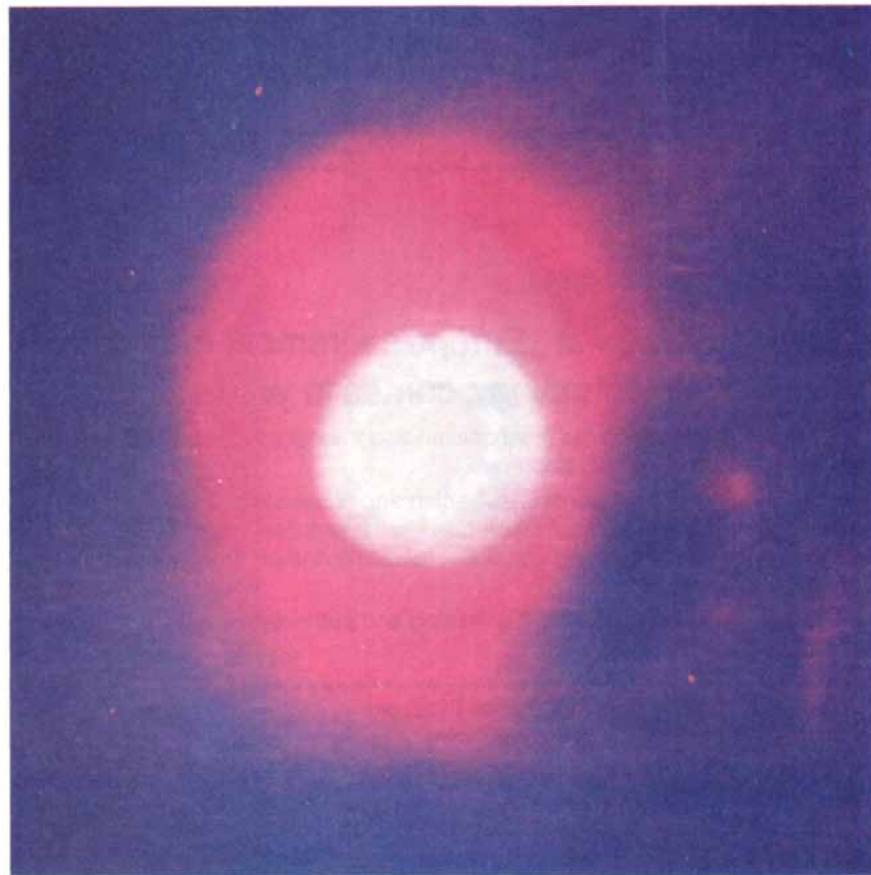
LASER-BEAM SPOT is seen as it appeared from the space shuttle Discovery during a tracking experiment conducted last June. An argon laser on a mountaintop in Hawaii projected the beam to the shuttle as the craft passed over the islands at an altitude of 230 miles. Initially pencil-thin, the beam widened to a diameter of 15 feet as it passed through the atmosphere. For more than two minutes the beam locked onto a retroreflector on the shuttle.
