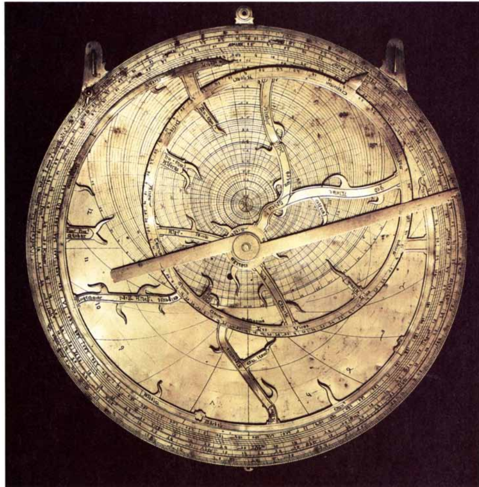
ASTROLABE simplified astronomical calculations, including the telling of time. Its nested brass plates are a projection of the celestial sphere onto two dimensions. The top plate, called the rete , is an open network of pointers indicating the positions of prominent stars. The off-center circle on the rete is the ecliptic. Under the rete is a solid plate on which is engraved a celestial coordinate system for a particular latitude: lines of equal altitude, lines of equal azimuth and hour circles. By turning the rete around the central pin, which represents the
