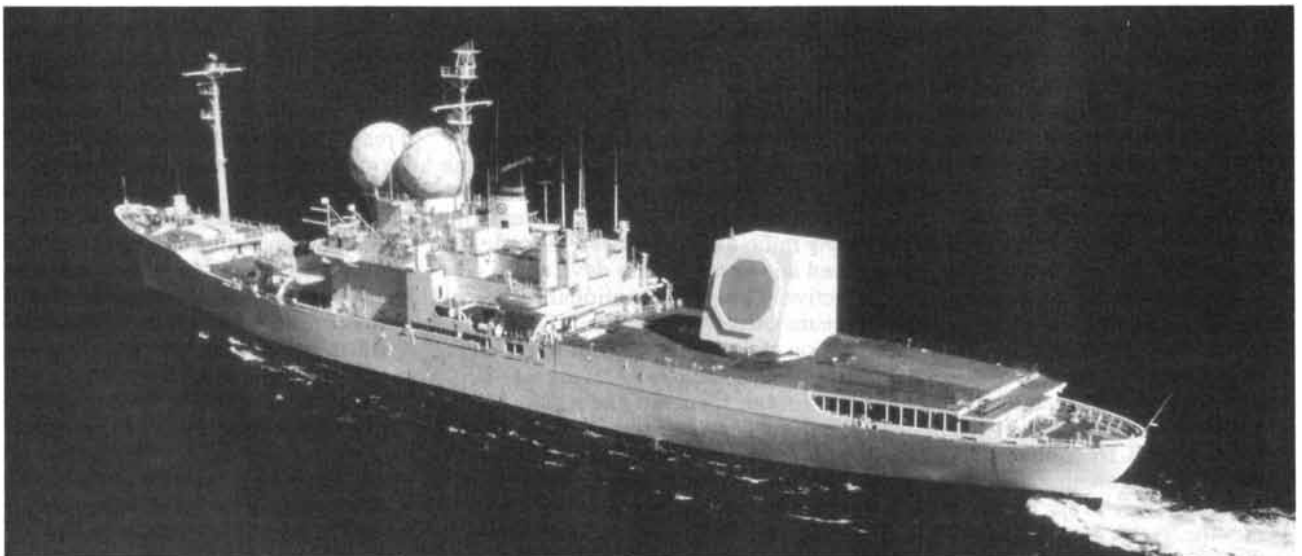
U.S. NAVY SHIP Observation Island has a COBRA JUDY phased-array radar mounted on the flat deck near its stern. The sophisticated radar collects intelligence data on flight tests of Soviet missiles.
