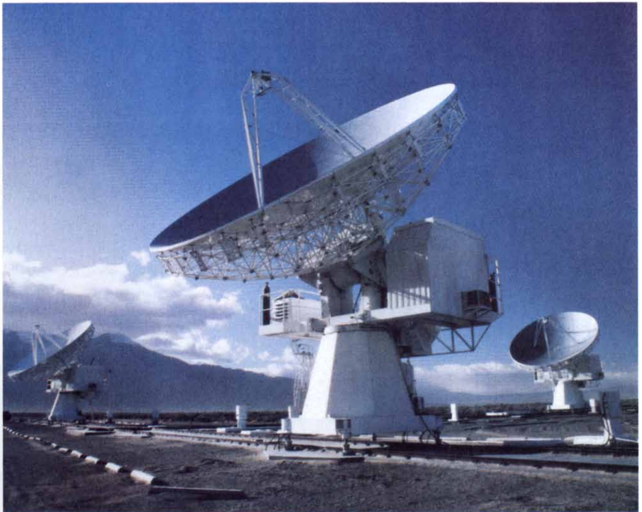
OWENS VALLEY INTERFEROMETER , which is operated by Caltech, consists of three millimeter-wave telescopes linked electronically. A superconducting tunnel detector is mounted on each
