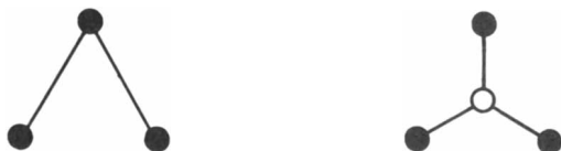
How a minimal spanning tree (left) is shortened if an extra point is allowed (right)
