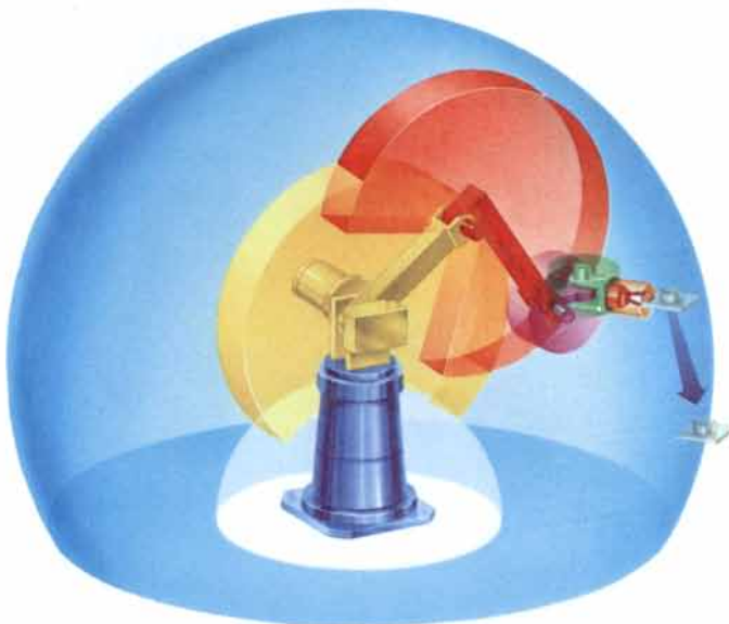
Figure 2: Three-dimensional illustration of the robot work cell layout, showing reach capability for the task in Figure 1. Areas of color show total reach as well as the joint limits stored in the robot model.
