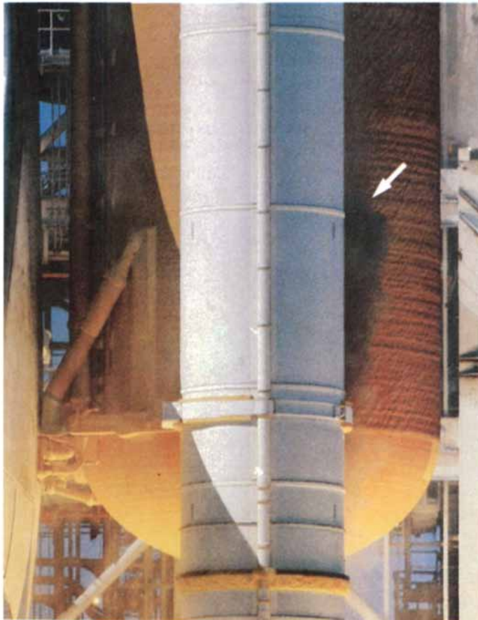
FAILURE of a seal doomed the space shuttle while it was still on the launch pad. Smoke leaked from the right-hand booster rocket and spurt-
