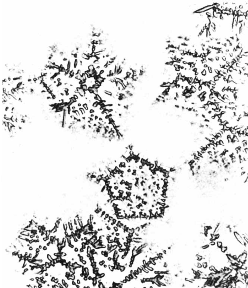
SHECHTMANITE "SNOWFLAKES" form when a molten alloy of aluminum and manganese is cooled rapidly. The "crystals" have the branched pattern of dendrites, or lobes, normally found in ice crystals, but because of the underlying icosahedral symmetry of shechtmanite, these samples have fivefold symmetry rather than the sixfold symmetry of ordinary snowflakes. The samples measure about 10,000 atomic spacings across and are magnified about 10,000 times in this electron micrograph, which was made in the laboratory of Leonid A. Bendersky and Robert J. Schaefer at the National Bureau of Standards.
