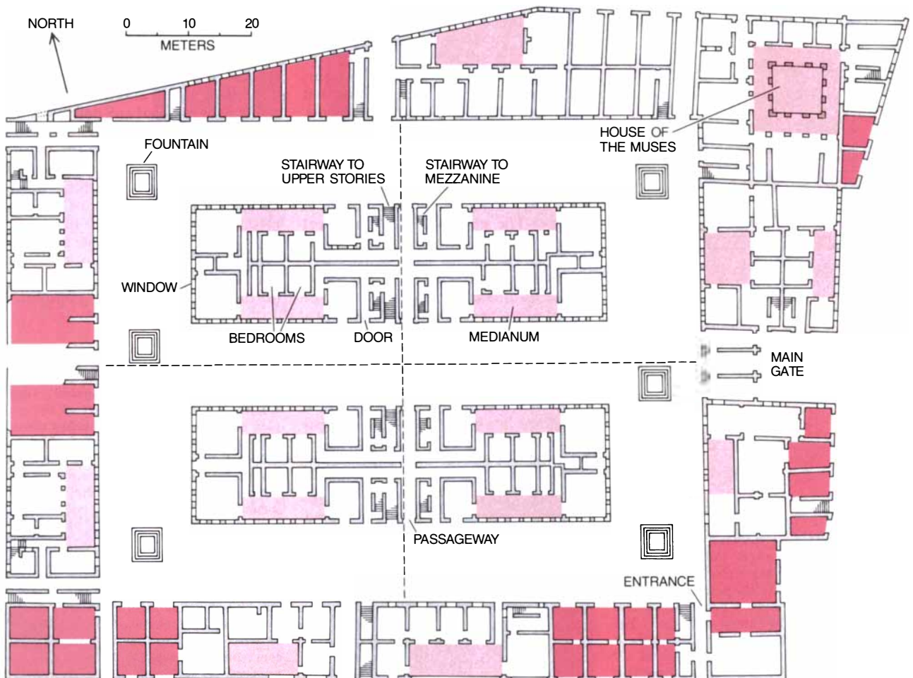
GROUND-FLOOR PLAN of the Garden Houses complex shows its basic geometry. The major east-west axis and the minor north-south axis cross at the center of the complex. The buildings were probably four stories high. Each of the 17 ground-floor apartments
