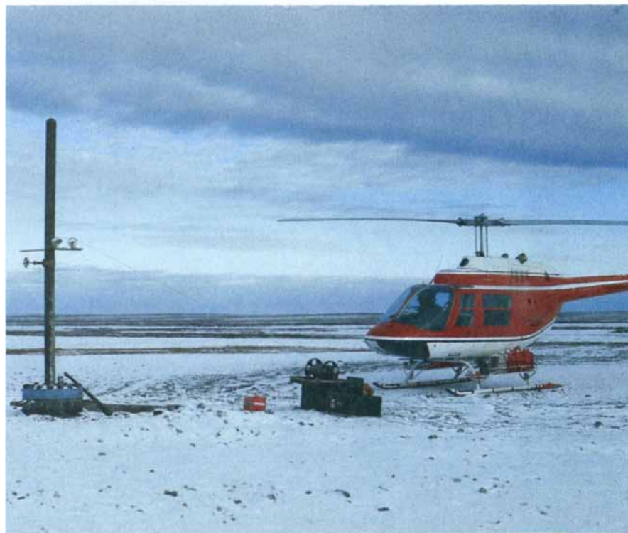
ABANDONED OIL WELL on Alaska's North Slope provides a way to measure temperatures in permafrost. Geophysicists fill wells with diesel oil and lower sensors into them.
