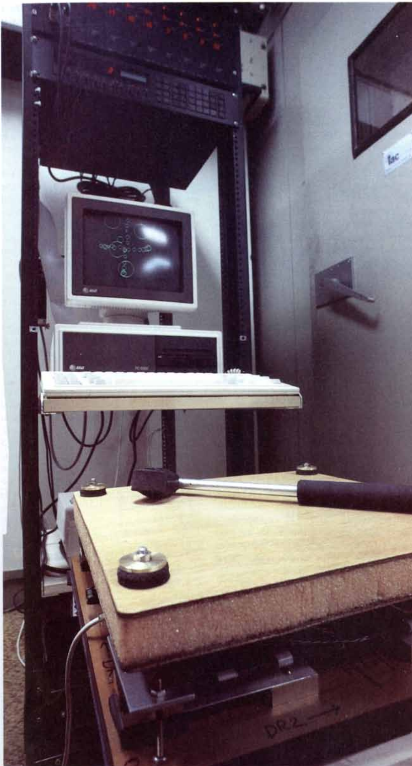
"INTELLIGENT" MUSICAL INSTRUMENT in the laboratory of one of the authors (Mathews) consists of a personal computer hooked up to a custom-made sensor and a commercially available digital sound synthesizer. The instrument enables one to "conduct" a programmed piece of music: tapping with a cushioned hammer on the rectangular "daton," or drum baton ( foreground ), sets the tempo; the placement of the hammer taps controls the instrumental balance and loudness. On the computer screen above the daton a series of strikes are displayed: a circle whose radius is proportional to the force of the strike indicates where the hammer hit the daton surface. The pair of black boxes on the rack above the computer are the sound synthesizer and a digital sound-processing device.
