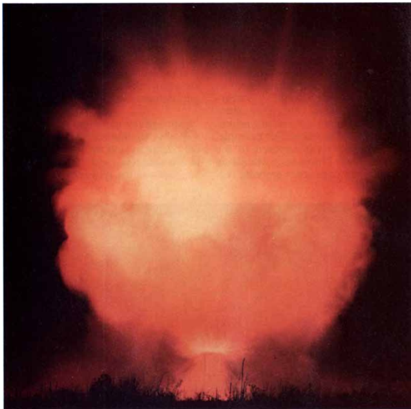
FIREBALL of a nighttime explosion of a 50-pound mixture of ammonium nitrate and fuel oil results from the afterburning of the explosion products; paraffin and sulfur have been added to the mixture to enhance the effect. The streaks at the base of the fireball are tracks made by turbulent burning during the expansion of the explosion-product gases.
