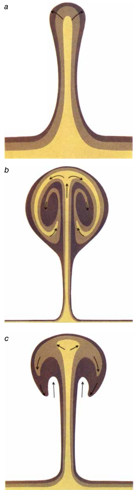
THREE TYPES OF BULB can be formed by the circulation associated with salt diapirs. If the sedimentary cover is softer (less viscous) than the salt, the diapir bulb is thumb-shaped (a); if the cover is stiffer, the bulb is balloon-shaped (b), and if the two layers are equally viscous, a mushroom-shaped bulb results (c). All three types of bulb can develop at depth, before the diapir encounters an upper boundary.
