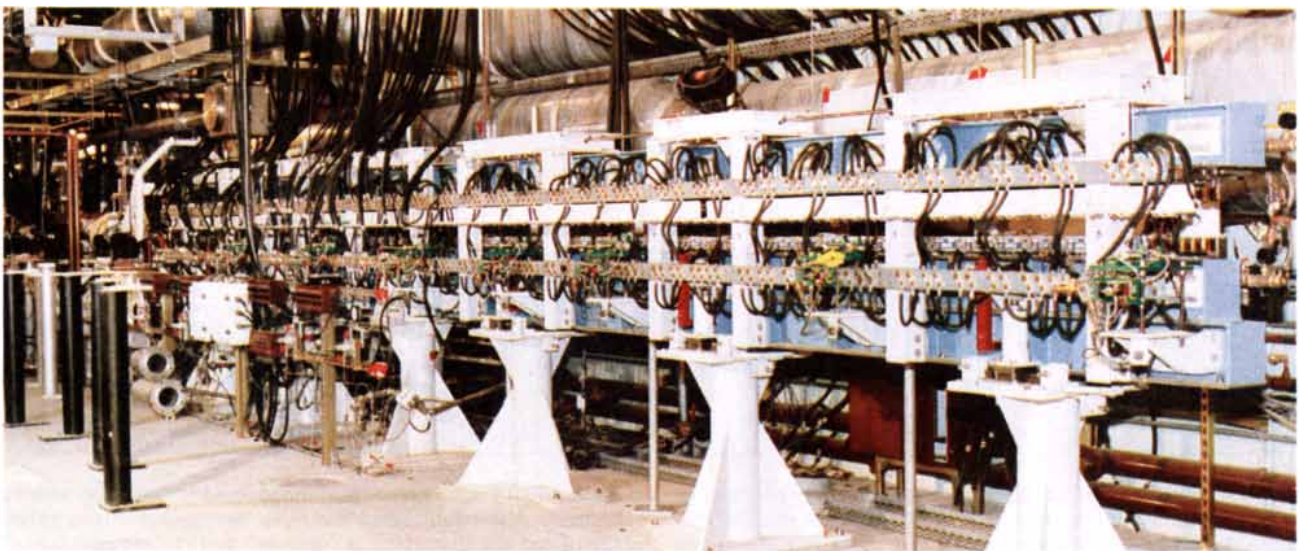
FREE-ELECTRON LASER called PALADIN at the Lawrence Livermore National Laboratory radiates in the infrared portion of the electromagnetic spectrum. A beam of electrons is accelerated
