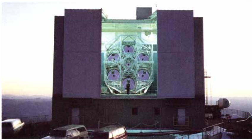
MULTIMIRROR TELESCOPE, operated by the Smithsonian Institution and the University of Arizona, is the first large telescope to use multiple primary mirrors and active optics.
