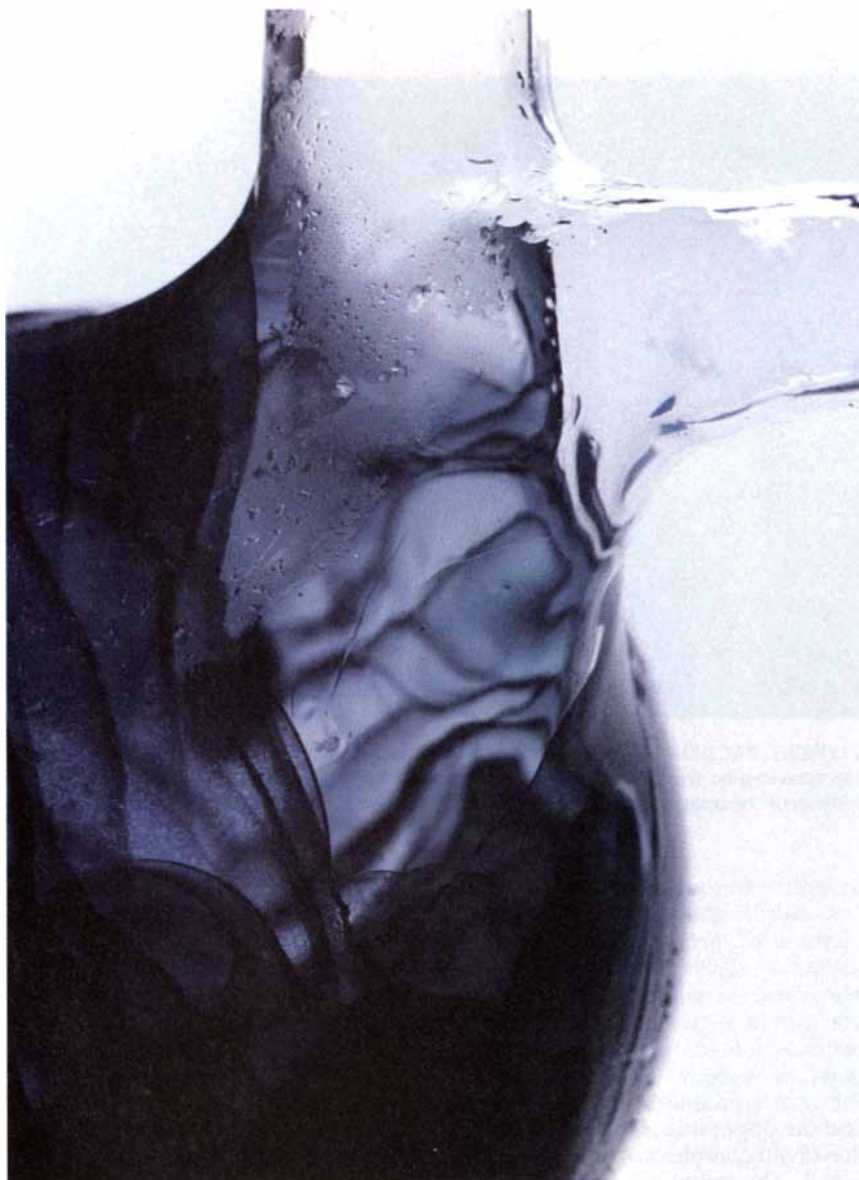
THIN FILM OF ELECTRIDER coating the inside of a flask appears blue when light is shined through it; this electrider absorbs red and infrared light. The optical absorbance of an electrider yields clues to how tightly the trapped electrons are held and how much they interact. The electrider in this photograph is made from cesium metal and crown-ether molecules called 18-crown-6; its structure is shown in the computer images on preceding pages. The film was made by Mark Kuchenmeister in the author's laboratory.
