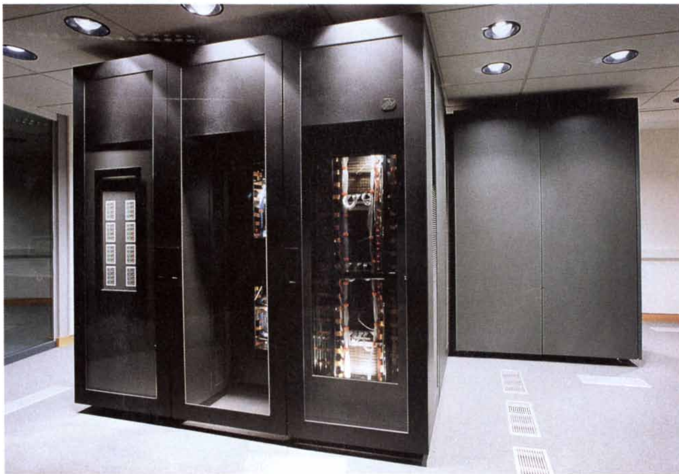
RP3, an IBM parallel computer test-bed, simulates various kinds of parallel architectures and challenges them with specific kinds of tasks. The effectiveness of an architecture for a particular task can be determined and the cost of a prototype avoided.
