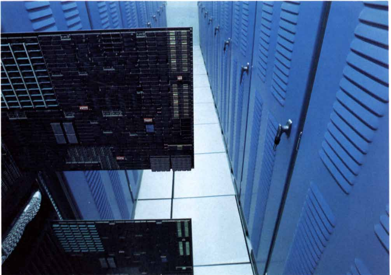
GF11, a scientific parallel processor capable of 11 billion floating-point operations per second, is being built by IBM Research.
