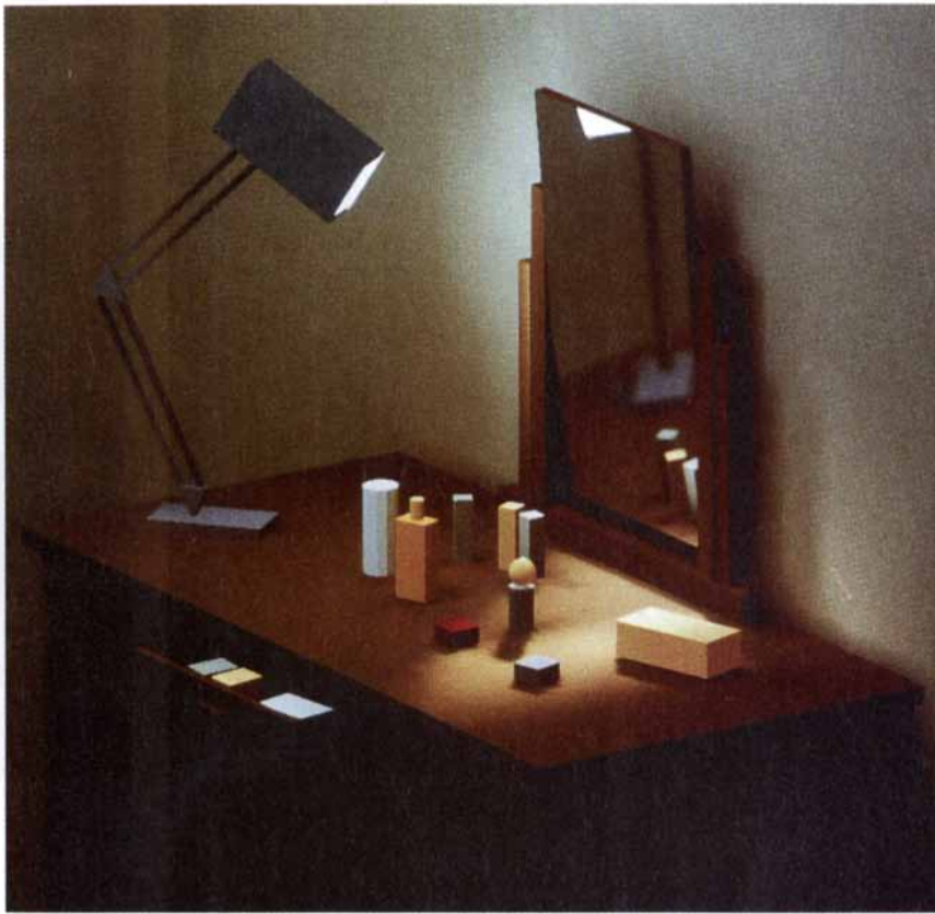
DRESSING-TABLE SCENE rendered at Cornell University shows the interplay of the specular reflections from the mirror and the diffuse reflections from dull surfaces.
