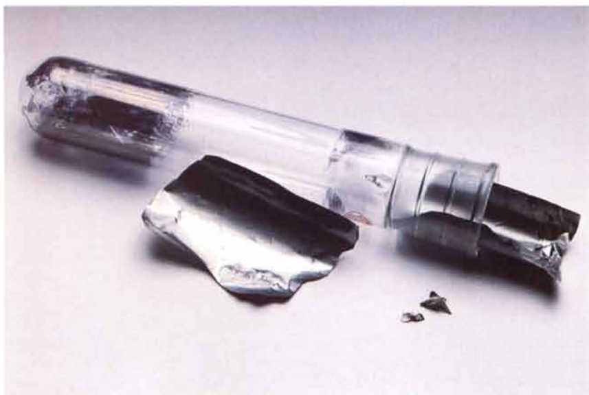
POLYACETYLENE SHEET is stripped from the walls of a reaction vessel after synthesis. As flexible as paper, the freestanding film must be doped to its conducting form.
